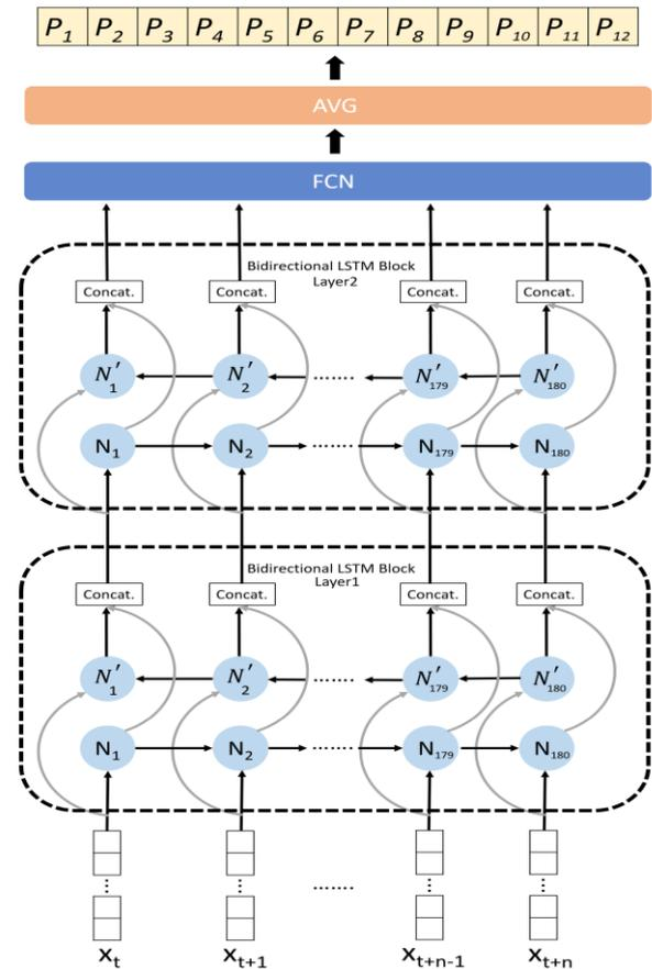
FIGURE 7. The architecture of LSTM model we used to compare.
