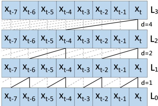
FIGURE 5. An example of dilated convolution while the kernel size is 2 and the delated size increases from 1 to 4 exponentially.
