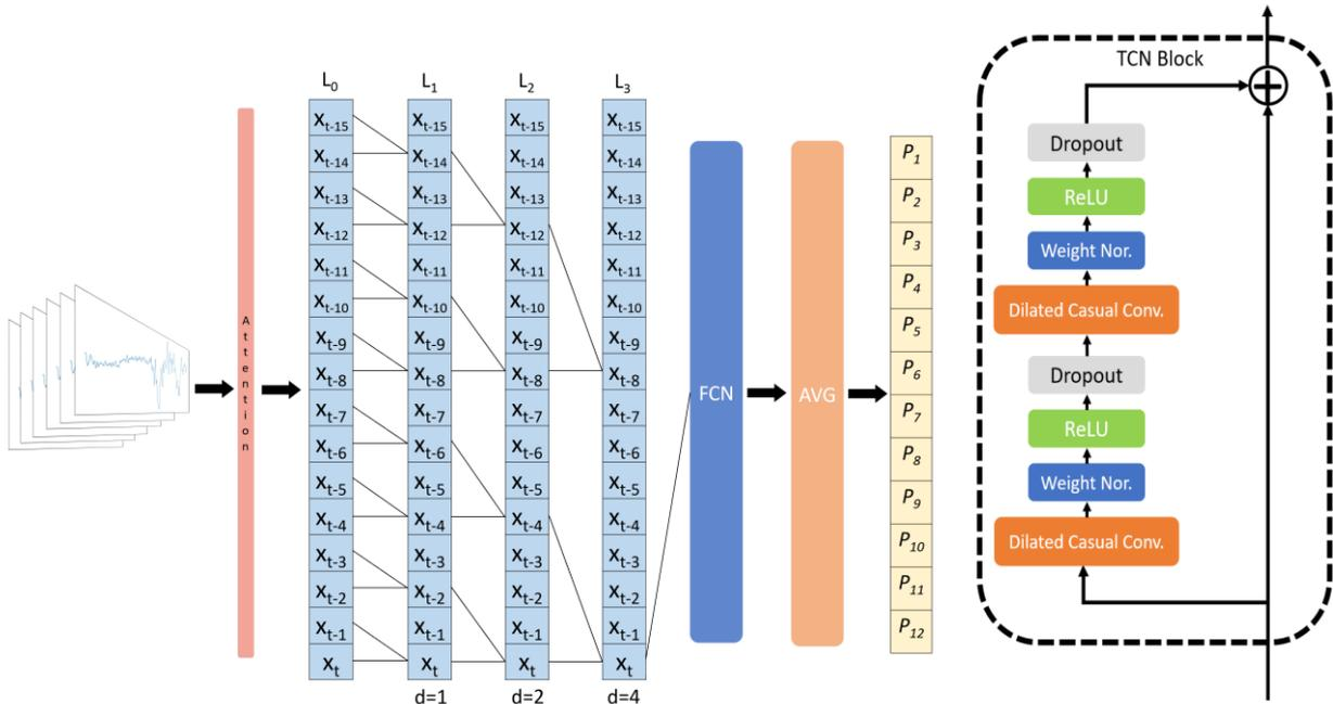
**FIGURE 3.** The architectural overall of our system in this paper. (a) An overview of the TCN model which give an example of kernel size = 2. The  $L_0$  represents the input after attention. The dilation size of  $L_1$ ,  $L_2$ , and  $L_3$  is 1,2, and 4, respectively. The output,  $P_1$  to  $P_{12}$ , is the probabilities of 12 classes. (b) A detail of each TCN layer.
