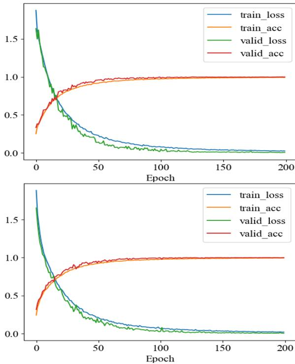
FIGURE 11. The loss and accuracy curve of one-layer attention. The curve above is applying attention before TCN and the curve below is applying after TCN.
