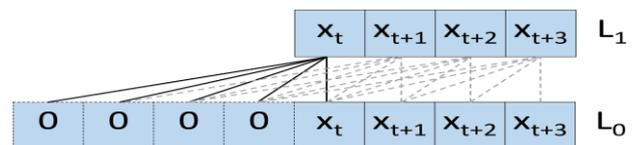
**FIGURE 4.** An example of 1D causal convolution while the kernel size is 5, the padding size is 4, and padding with 0.
