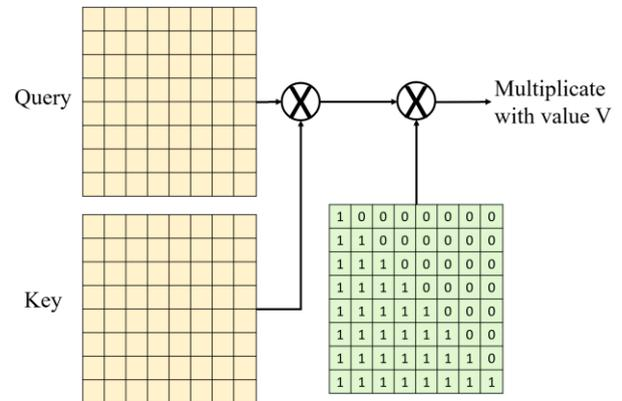
FIGURE 6. An example of the lower triangular function.
