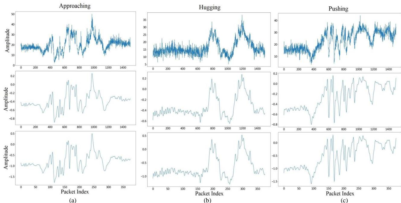
**FIGURE 2.** The flowchart of our methods. (a) is the amplitude data of interaction “Approaching”, (b) is the amplitude data of “Hugging”, and (c) is the amplitude data of “Pushing”. For the figures in first row, they represent the raw data. For the figures in middle row, they represent the data after a Butterworth lowpass filter and normalization. For the figures in third row, they represent the data after applying 1D DWT twice. As you can see, the length of packets in third row is 375.
