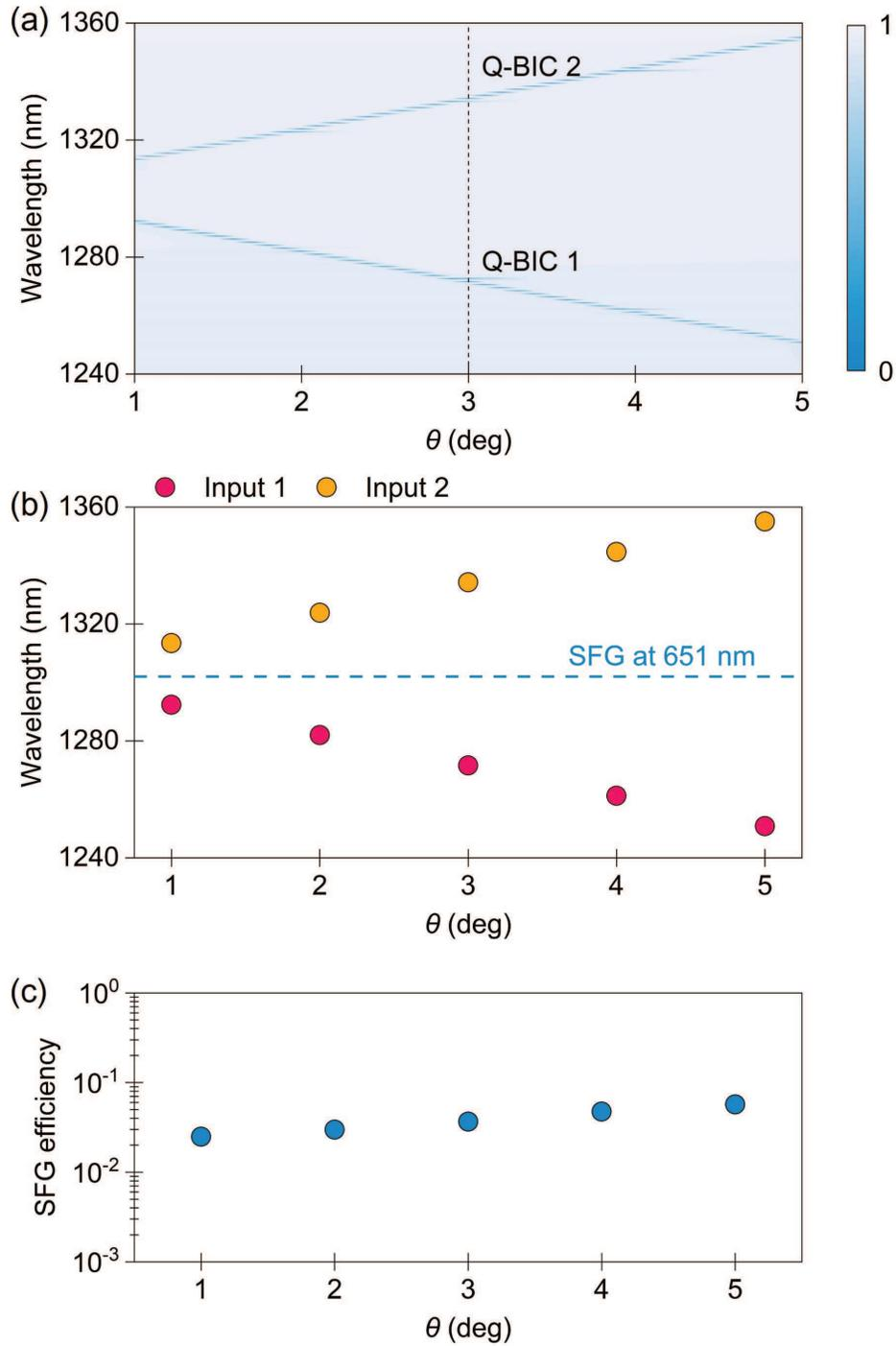
FIG. 6. (a) The evolution of transmission spectra of the resonant grating waveguide structure as a function of the incident angle  $\theta$ . (b) The fixed SFG wavelength of 651 nm when the wavelengths of the two input beams are jointly tuned by selecting  $\theta$ . (c) The SFG conversion efficiency as a function of  $\theta$  at the corresponding quasi-BICs.
