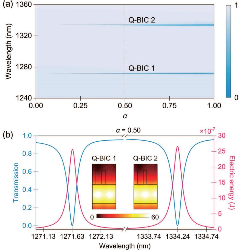
FIG. 2. (a) The evolution of transmission spectra of the resonant grating waveguide structure as a function of the grating geometry parameter  $\alpha$  under oblique incidence  $\theta = 3^\circ$ . (b) The transmission spectrum and electric energy inside the  $\text{LiNbO}_3$  waveguide layer around the dual quasi-BICs with  $\alpha = 0.5$ . The inset shows electric field distributions at the resonance wavelengths.
