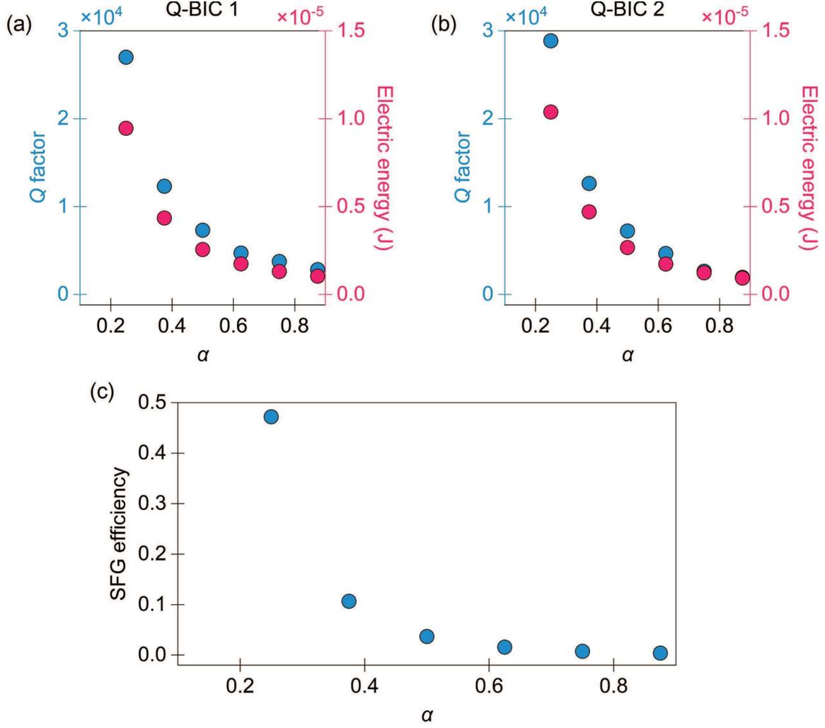
FIG. 4. (a) and (b) The  $Q$  factor and electric energy inside the LiNbO<sub>3</sub> waveguide layer as a function of the grating geometry parameter  $\alpha$  at the quasi-BICs. (c) The SFG conversion efficiency as a function of  $\alpha$  at the quasi-BICs.
