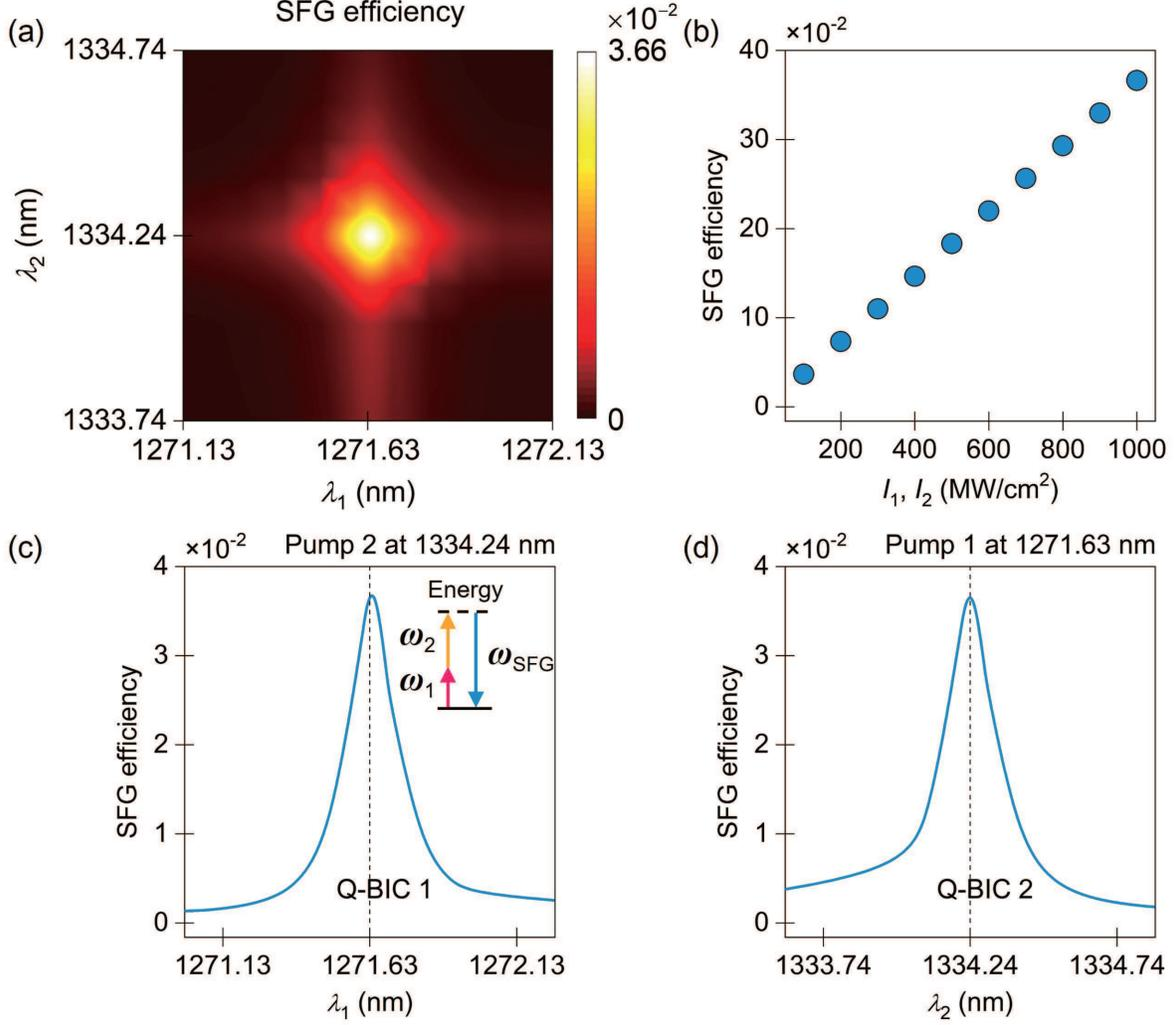
FIG. 3. (a) The SFG conversion efficiency as a function of the two input wavelengths around the quasi-BICs. (b) The SFG conversion efficiency as a function of the input intensity. (c) and (d) The SFG conversion efficiency as a function of the input beam 1(2) wavelength when the input beam 2(1) wavelength is kept constant at quasi-BIC 2(1).
