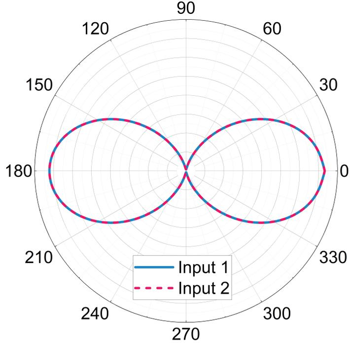
FIG. 5. The polar plots for the SFG conversion efficiency as a function of the polarization angle of the input beam 1(2) when maintaining fixed polarization of the input beam 2(1) along the  $z$ -axis. In both plots,  $0^\circ$  and  $90^\circ$  represent polarizations along the  $z$ - and  $x$ -axis, respectively. The SFG efficiencies are normalized to the maximum.
