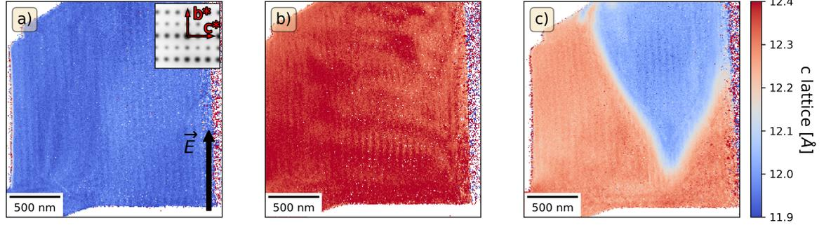
Figure S 7. The real space maps of the  $c$  lattice parameter when applying field along the  $b$  axis [corresponding to Fig. 2(a) (main text) and Fig. S1(b)] **(a)** before applying an electric field of the sample with  $E$ -field along the  $b$  axis **(b)** The real space map of the  $c$  lattice parameter while applying the maximum electric field **(c)** The real space map of the  $c$  lattice parameter after quenching the specimen back to 0V.
