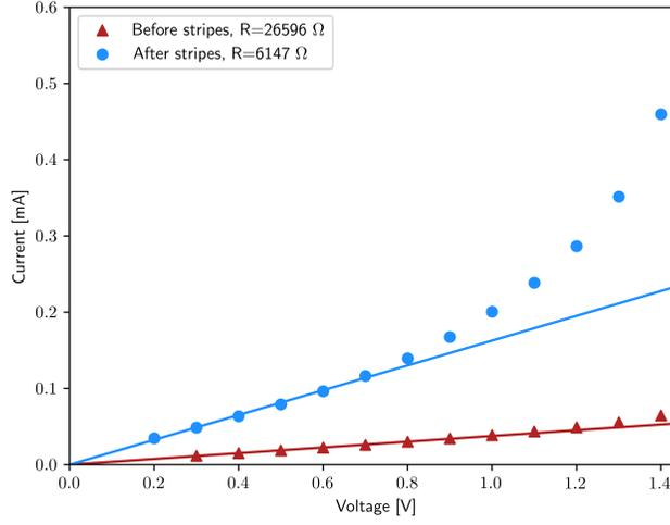
Figure S 9. Current-voltage (I-V) curves of the sample with a contact configuration as in Fig. S1e. The measurement is performed before (triangle) and after (circle) establishing the stripe phase corresponding to the pattern in Figure 3g of the main text. The amplitude of the resistance extracted from the linear regime is also reported in the label.
