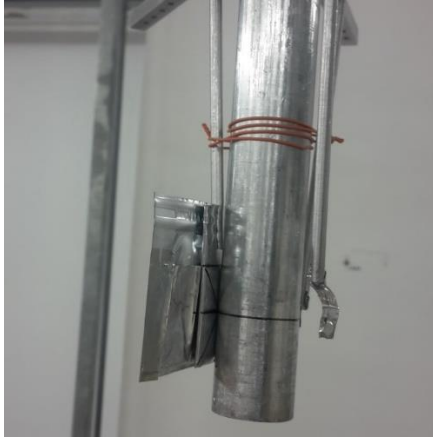
Figure 1: Lutetium foil irradiation setup.
