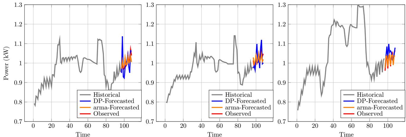
Fig. 3. ARMA forecasts of power demands of three houses, where the accuracy of DP-Forecasting is 0.45, i.e.,  $\rho = 0.45$  and  $(\epsilon, \delta) = (0.8, 0.5637)$ .
