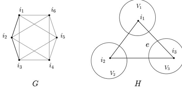
Figure 1: Lifting a graph  $G$  into a hypergraph  $H$  when  $t = 3$ : We depict a 4-connected ring base graph  $G$  on the left and a single edge in the hypergraph  $H$  on the right.  $(i_1, i_2, i_3)$  forms an hyperedge  $e$  in  $H$  if and only if  $(i_1, i_2, i_3)$  is a walk in  $G$ .
