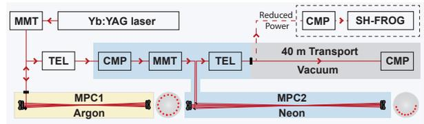
Figure 2: Experimental setup used for post-compression comprising two gas-filled MPC stages (MMT: Mode-matching telescope, TEL: Telescope, CMP: Compressor), a pulse diagnostics section and a 40 m long beam, transport section to an application area. The beam patterns obtained at the MPC mirrors are indicated schematically for both cells.
