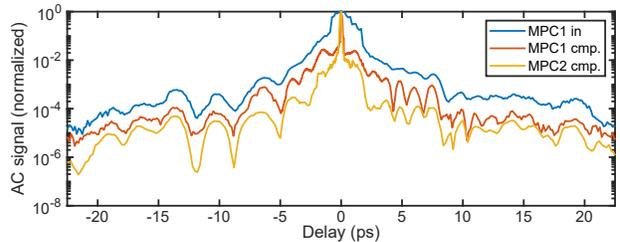
Figure 4: Third-order autocorrelation (AC) traces measured at the output of the laser and after first and second compression stage.
