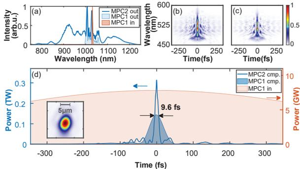
Figure 3: (a) Measured spectra at input and output of MPC1 and output of MPC2. (b) and (c) show recorded and retrieved FROG traces of the MPC2 compressed output respectively. (d) MPC1 and MPC2 compressed output pulses retrieved using FROG. The figure also highlights the peak power enhancement from MPC1 input to MPC2 compressed output. Inset: Beam profile after focusing the compressed output of MPC2 reaching a spot size of  $4.5 \mu\text{m} \times 3.9 \mu\text{m}$ .
