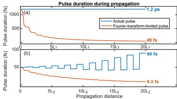
Figure 1: Simulated post-compression using a two-stage cascaded MPC setup. Panels (a) and (b) show the pulse duration and corresponding FTL during propagation in the first and second cell in units of cell lengths  $L_{1,2}$ , respectively.
