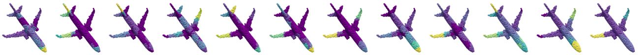
FIGURE 5. Attention Visualization of the classification token for each block (1-12), averaged across heads for a finetuned model without pretraining. It is evident the locations it attends to do not follow any recognizable pattern. In each layer, the attention is focused on a specific location, which is often the same between layers (e.g. head in layers 0,5,7,10).
