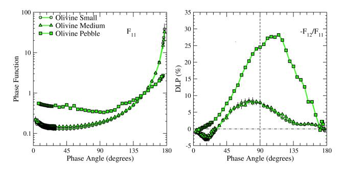
Figure 3. Phase function (left) and degree of linear polarization (right) of the olivine samples. The phase functions are normalized to 1 at 150 degrees.
