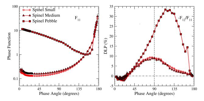
Figure 4. Phase function (left) and degree of linear polarization (right) of the spinel samples. The phase functions are normalized to 1 at 150 degrees.
