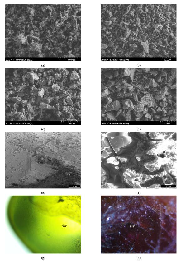
**Figure 1.** FSEM micro-photographs of the *Olivine Small* (a), *Spinel Small* (b), *Olivine Medium* (c), *Spinel Medium* (d), *Olivine Pebble* (e), *Spinel Pebble* (f). Optical microscopy images of the *Olivine Pebble* and the *Spinel Pebble* are also shown in panels g and h, respectively.
