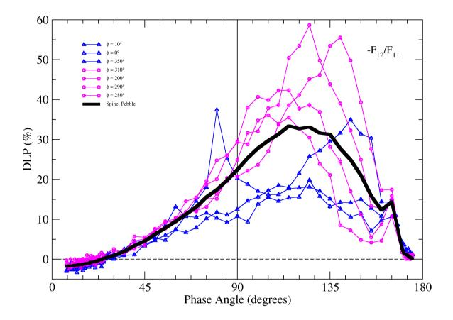
Figure 5. Phase-angle dependence of the degree of linear polarization of the Spinel Pebble. Each curve corresponds to a different orientation of the grain. The blue triangles correspond to sharp-cornered sides, whereas the magenta circles to smooth faces. The black line is the average curve for the Spinel Pebble.
