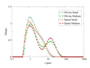
Figure 2. Size distribution of the four powdered samples.
