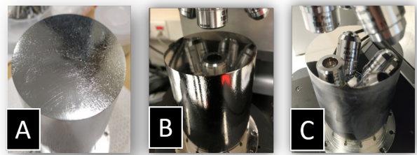
Figure 6: Visual inspection of the QPR sample: a) after BCP, b) after EP, c) after MP.
