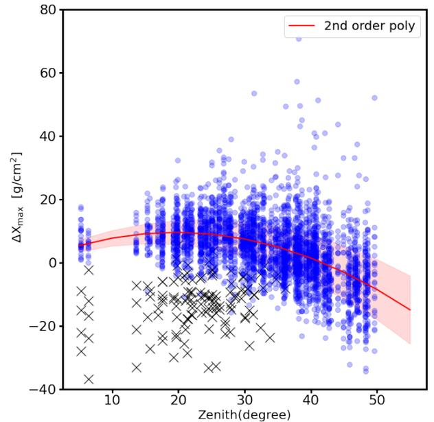
FIG. 7: Zenith angle distribution of  $\Delta X_{\max}$  of the showers shown in Fig. 6. The black crosses are showers having distance to  $X_{\max}$  lower than 3 km and are excluded from the fit. The red line is a  $2^{\text{nd}}$  degree polynomial fit to the showers with the dashed line showing the  $1\text{-}\sigma$  deviation. The fit coefficients are shown in Table II.
