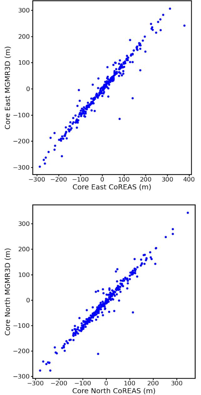
FIG. 12: Correlation in reconstructed cores for all showers between CoREAS and MGMR3D for two directions .
