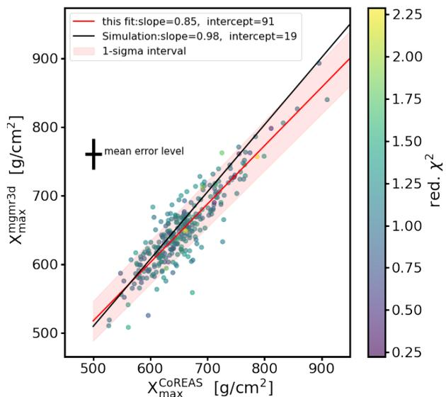
FIG. 10: Reconstructed  $X_{\max}$  with MGMR3D and LOFAR. The  $X_{\max}$  values reconstructed with MGMR3D are corrected with the zenith correction from Table II. The mean error bar is shown by the black cross. The red line is the fit to the data points considering the vertical mean error in the fit. The shaded area is the 1- $\sigma$  interval of the fit. The black line corresponds to the prediction from simulation as discussed in Section IV B.
