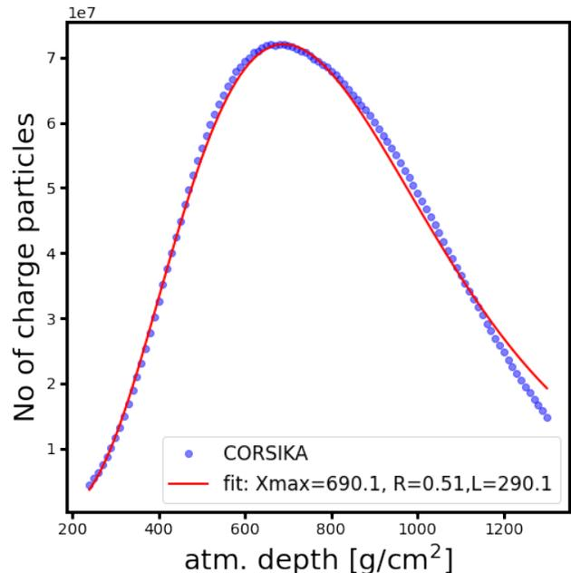
FIG. 9: Longitudinal profile for a simulated shower. This is one of the extreme cases shown in Fig. 8. The dots are the CORSIKA values and the line is fit to the profile.
