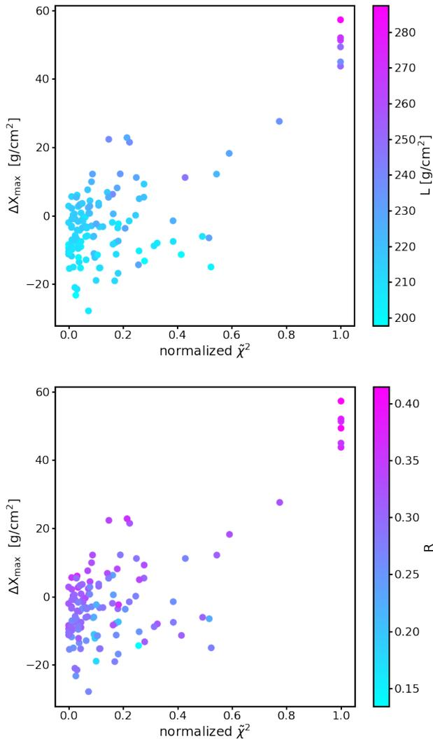
FIG. 8:  $\Delta X_{\max}$  as function of  $\tilde{\chi}^2$  with colorbars indicating true  $L$  (top) and  $R$  values (bottom) for an ensemble of proton simulations for a subset of showers. The  $\tilde{\chi}^2$  values are normalised between 0 to 1 individually for each set of simulated showers.
