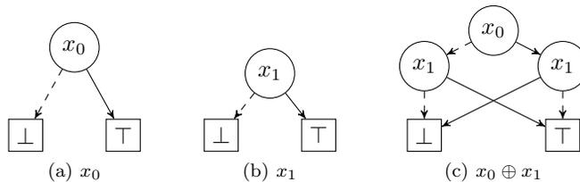
Figure 2: Examples of Reduced Ordered Binary Decision Diagrams. Terminals are drawn as boxes with the Boolean value and BDD nodes as circles with the decision variable. *Low* edges are drawn dashed while *high* edges are solid.
