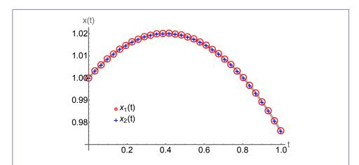
Figure 3 The forward  $\mathbf{x}_1(t_1)$  (red circles) and backward  $\mathbf{x}_2(t_2)$  (blue crosses) degrees of freedom obtained from the critical point of  $\mathbb{E}^{\lim}_{\mathrm{IVP}}$  with  $V(x)=\alpha x$ . We discretize with  $N_{\gamma}=32$  points and the SBP21 operators. The trajectory from a LSODA solver of the corresponding equation of motion is given as gray solid line.
