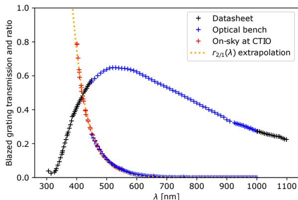
**Fig. 21.** First diffraction-order transmission of the blazed Thorlabs grating with 300 lines/mm (blue and black) and the ratio of transmissions of the order 2 over the order 1 (red, blue, and orange).
