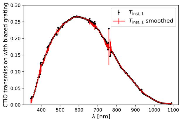
**Fig. 24.** Measured  $T_{\text{inst},1}(\lambda)$  curve for the CTIO 0.9 m telescope equipped with a Thorlabs 300 lines/mm blazed grating (black points) from a photometric night. The red curve is a smoothing using a Savitzky–Golay filter of order 1 and a window size 17.
