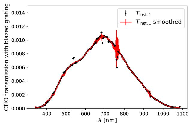
**Fig. 26.** Measured  $T_{\text{inst},1}(\lambda)$  curve for the CTIO 0.9 m telescope equipped with an amplitude holographic grating of about 350 lines/mm (black points) from a photometric night. The red curve shows a smoothing using a Savitzky–Golay filter of order 1 and a window size 11.
