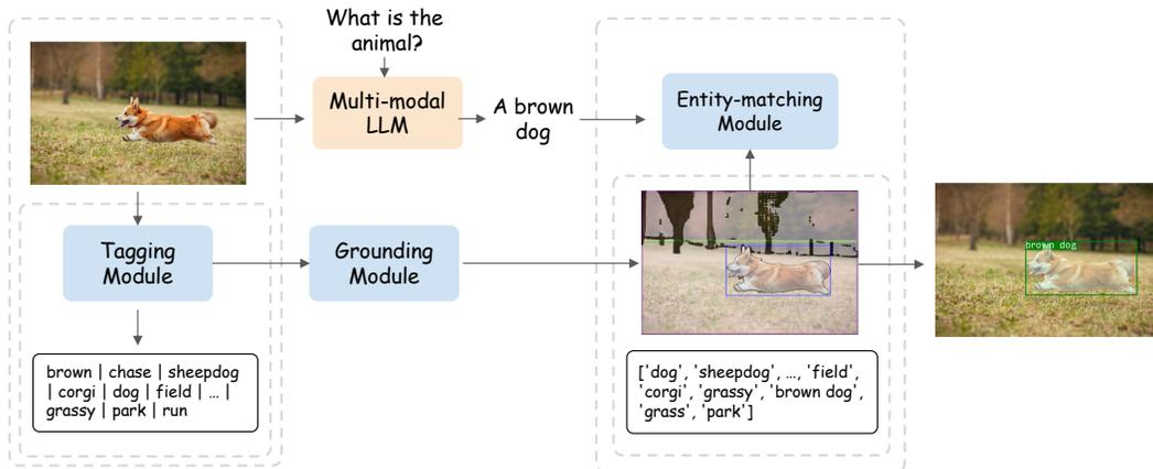
Figure 2: The pipeline of visual grounding that is composed of a tagging module, a grounding module and an entity-matching module.
