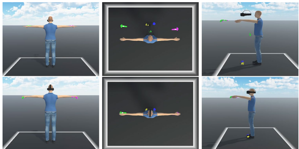
Fig. 9 In the top row, the user is well positioned according to the front view but in the top view he is in front of the avatar, this generates a misalignment and the arms are not able to reach the controllers. In the bottom row, the alignment is correct
