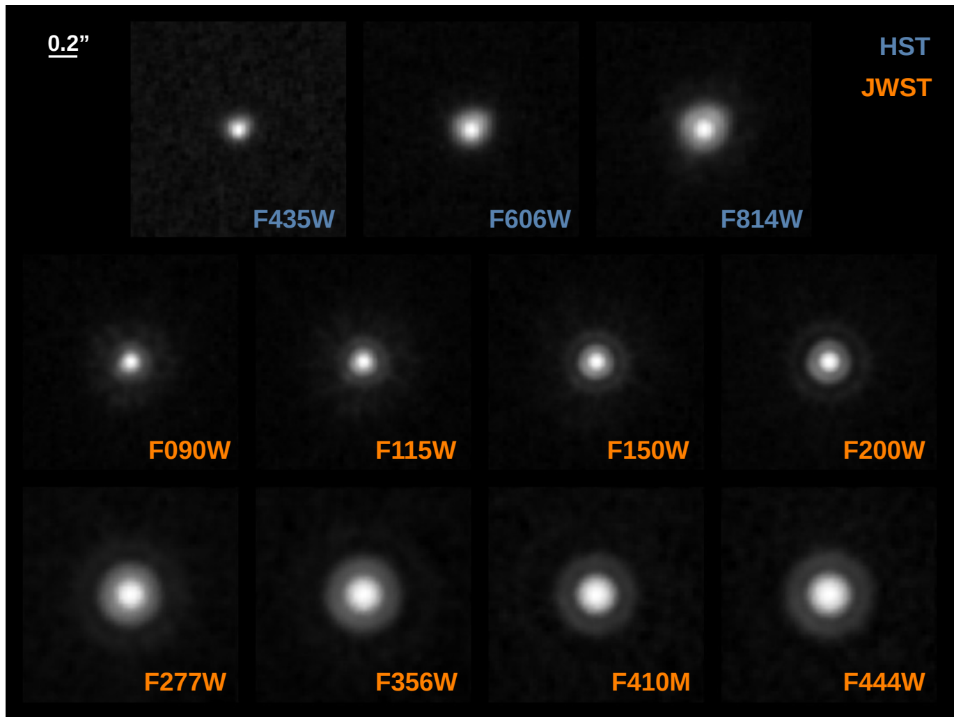
Fig. A.1. Stacked signal of six unsaturated stars in the same field in different bands and after coadding all three epochs (for JWST). The stars have been aligned before stacking using steps of 3 mas. In order to better show the sidelobes and diffraction spikes, we plot the logarithm of the stacked signal. The stacked signal is used as a model for the PSF in each filter.
