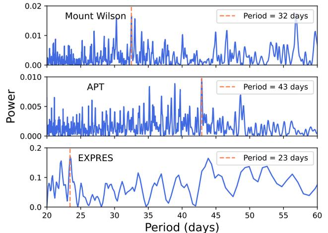
**Figure 3.** Periodogram created by chromospheric data from the Mount Wilson Observatory HK Project, photometric data from the Automatic Photoelectric Telescope at the Fairborn Observatory, and RV data from EXPRES. The red line shows the rotation period of the star at 32 days (MWO), 43 days (APT), and 23 days (EXPRES).
