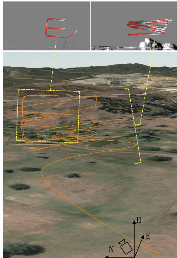
Fig. 14. Example of the estimated trajectory by our AEB tracker and the 3D GPS trajectory in a 3D plot. The first row shows the estimated trajectory (marked by red dots) of the tracked quadrotor overlaid on the event reconstruction frames. The second row shows the 3D GPS data of the full trajectory. The camera position and East-North-Up direction are marked at the bottom.
