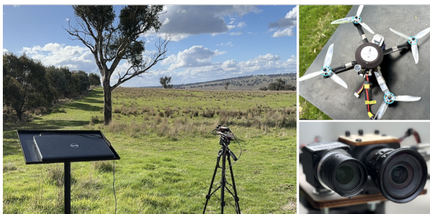
Fig. 13. Left: outdoor flying quadrotor experiments. Right: Our quadrotor with an RTK-GPS and our stereo event-frame camera.
