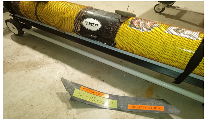
(b) Bent wing and cut netting upon recovery.
