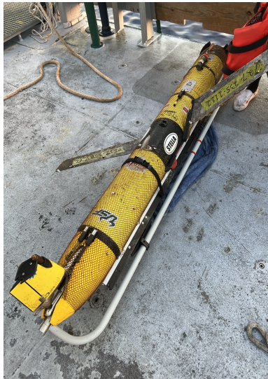
Fig. 24: Broken support rails of USF-Stella.
