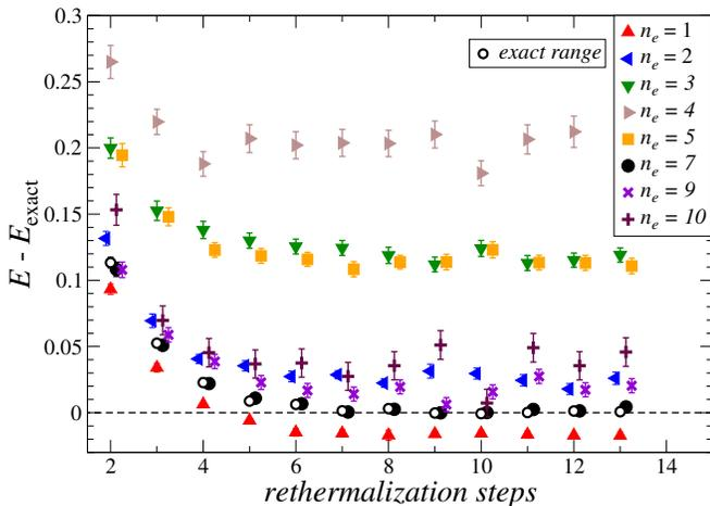
FIG. 3. Energy discrepancy for the QMS algorithm with inexact QPE grid with fixed extrema  $[-1.1, 3.1]$  (in units of  $J$ ) at  $\beta J = 0.25$ .
