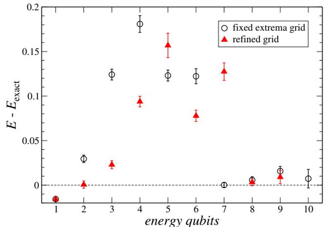
FIG. 4. Effects of the two grid prescriptions for the QMS algorithm on energy discrepancies with inexact QPE grids at  $\beta J = 0.25$  and with 10 rethermalization steps.
