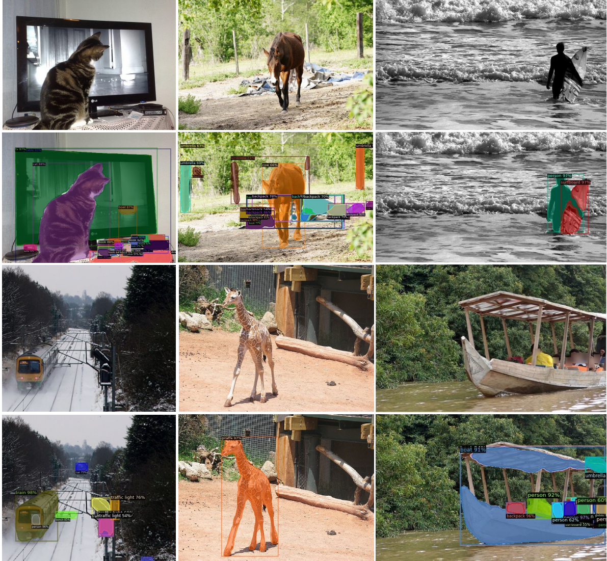
Figure 7. Illustration of predictions obtained with model trained on COCO with only 0.4% of labels. The model uses a DINOv2 [22] backbone and achieves an AP of 31.0, which is superior to what the previous SOTA achieved using 25x more labels (PT achieves 30.8 AP with 10% of labels).
