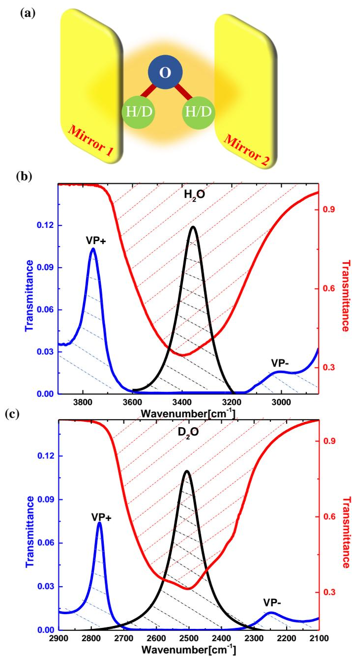
**Figure 1.** (a) Schematic representation of an FP cavity containing water/heavy water molecule. (b) 7<sup>th</sup> and (c) 5<sup>th</sup> mode of the cavity (black trace) is coupled to OH/D stretching band of H<sub>2</sub>O/D<sub>2</sub>O (red trace) resulting in the formation of vibro-polaritonic states (VP+ and VP-; blue trace).
