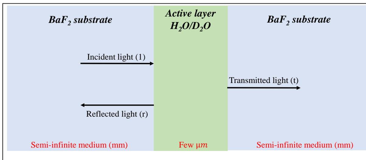
**Figure S1.** Schematic representation of the non-cavity structure used for modelling in transfer matrix methods (TMM) simulation.
