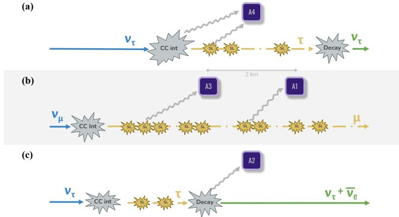
**Figure 1:** Cartoons of cascades from multiple particles in the same event triggering one station (a), cascades from multiple stochastic losses (SL) from the same muon track triggering two different stations (b), and a decay from a tau particle triggering one station (c). Outgoing neutrinos from tau decays are depicted in green though they are unlikely to be observed.
