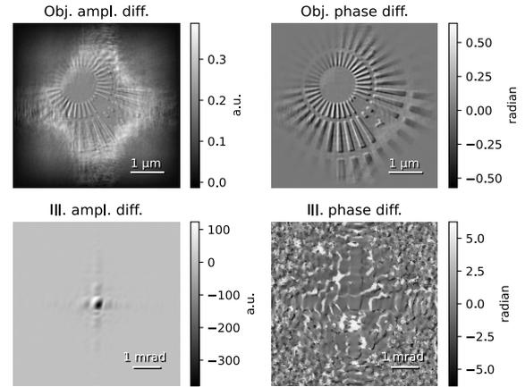
**Fig. 12.** Amplitude and phase difference between the final result of Figure 10 and the reference result (Figure 5). The amplitude of the object is higher, while the amplitude of the illumination is lower. The contour line around the sharp features of the object phase indicate a small shift relative to the reference result.
