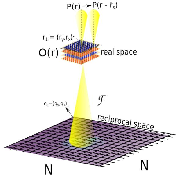
**Fig. 1.** Schematic setup for far field ptychography. The illumination is localized and scanned over the object  $O(r)$ . The detector captures the transmitted beam in the far field for each scan position. Illustration based on (Bangun et al., 2022).
