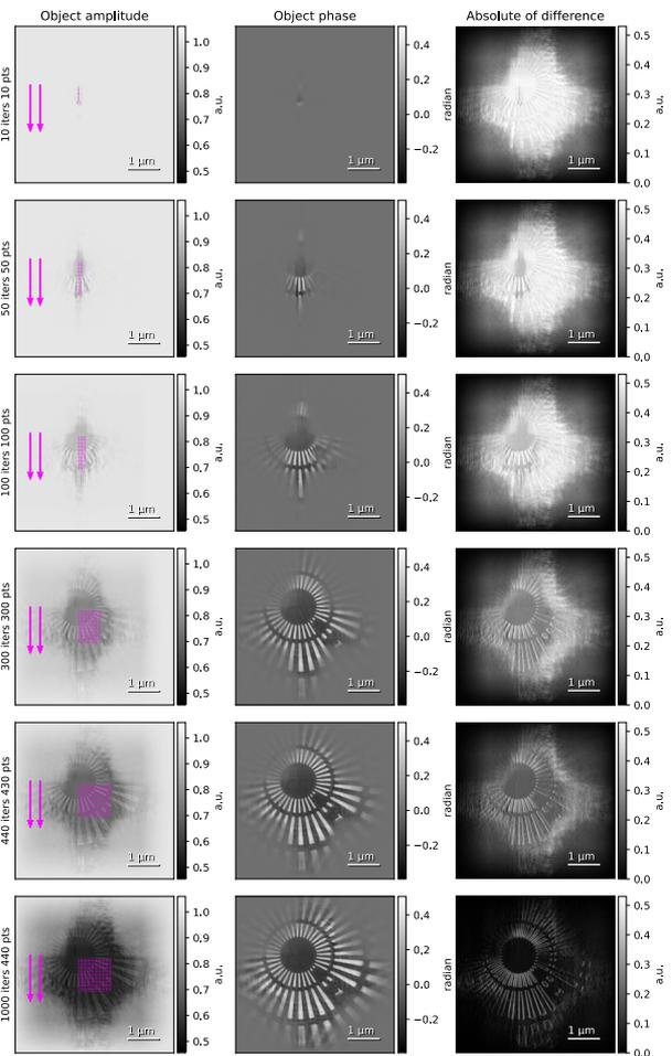
**Fig. 6.** Simulated live reconstruction following the original line scan pattern in  $y$  direction. The magenta dots in the left column indicate the scan positions. The right column shows the absolute value of the difference to the reference result.
