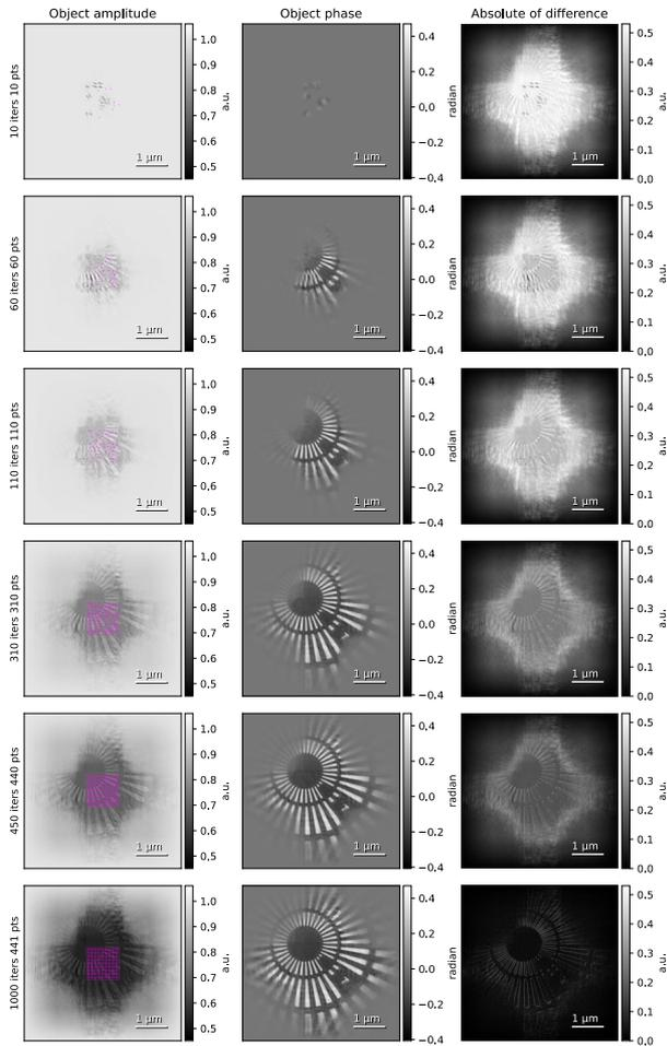
**Fig. 7.** Simulated live reconstruction with a random scan pattern. The magenta dots in the left column indicate the scan positions. The right column shows the absolute value of the difference to the reference result.
