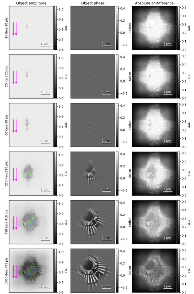
**Fig. 10.** Simulated parallelized live reconstruction on four gradually growing disjoint subsets. The colored dots in the left column indicate the scan positions, with the color indicating the subset. The right column shows the absolute value of the difference to the reference result.
