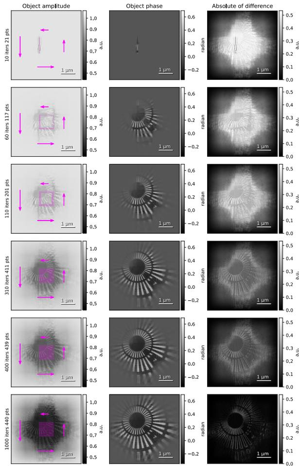
**Fig. 8.** Simulated live reconstruction following a spirangle scan pattern. The magenta dots in the left column indicate the scan positions. The right column shows the absolute value of the difference to the reference result.
