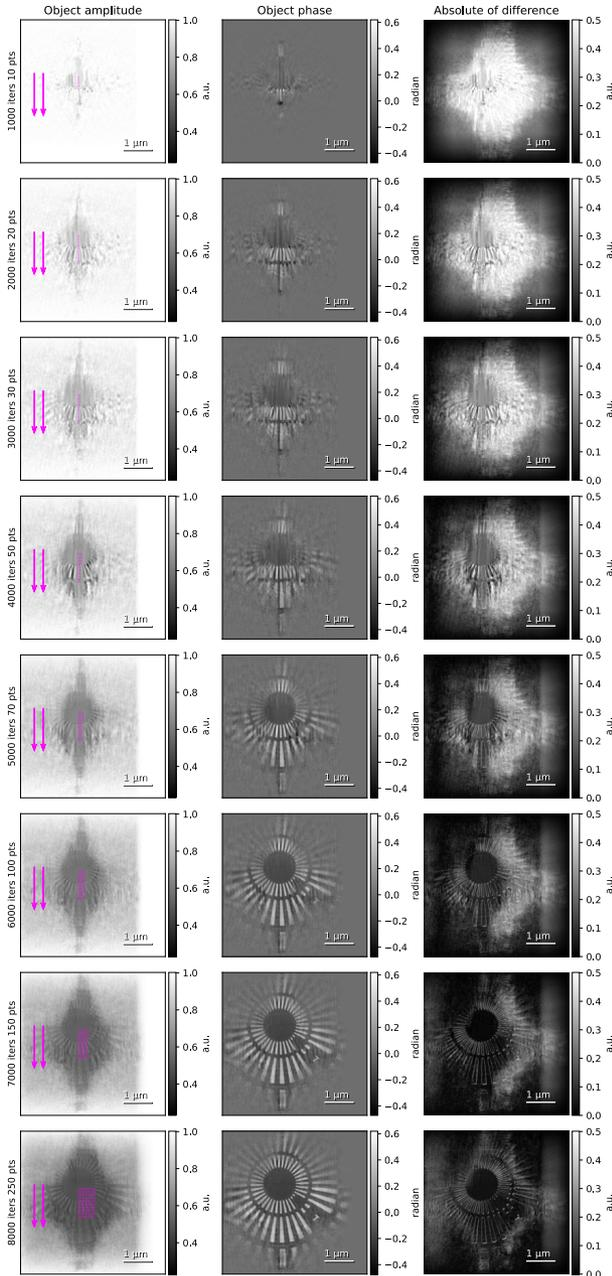
**Fig. 11.** Simulated live reconstruction following the original line scan pattern in  $y$  direction with over-optimization on a small subset of input data. The magenta dots in the left column indicate the scan positions. The right column shows the absolute value of the difference to the reference result.
