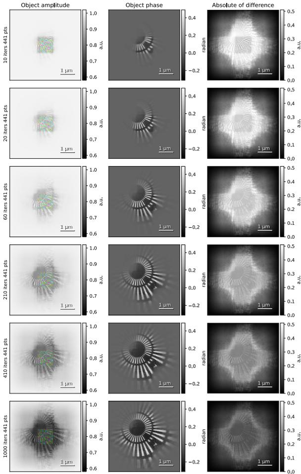
**Fig. 9.** Simulated parallelized reconstruction on four random disjoint subsets. The colored dots in the left column indicate the scan positions, with the color indicating the subset. The right column shows the absolute value of the difference to the reference result.
