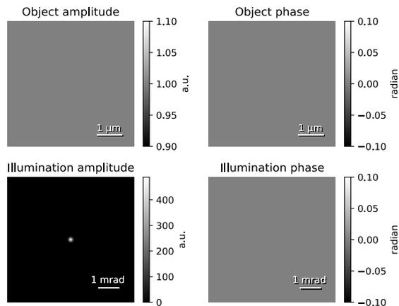
**Fig. 4.** Starting value for all simulated live reconstructions. The object is initialized with the identity function. The illumination amplitude is initialized with a small Gaussian peak and flat phase of 0.
