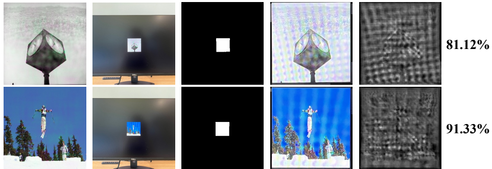
Figure 16: Examples of decoding under severe moire distortions. Each column shows original encoded images, physical photographs, localization masks, cropped images, decoded patterns, and the corresponding BER.
