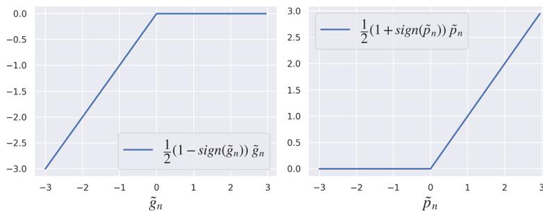
**Figure 5** An illustration of the sign-based function depending on gap  $g_n$  and contact pressure  $p_n$
