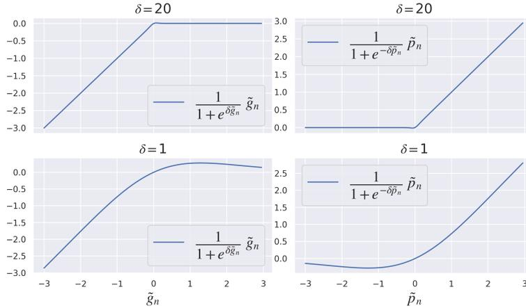
**Figure 6** An illustration of the Sigmoid-based function depending on gap  $g_n$  and contact pressure  $p_n$  for different  $\delta$  values.
