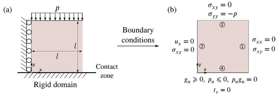
**Figure 11** Contact problem between an elastic block and a rigid flat surface, (a) geometry, supports and loading, and (b) an equivalent system including all relevant boundary conditions.
