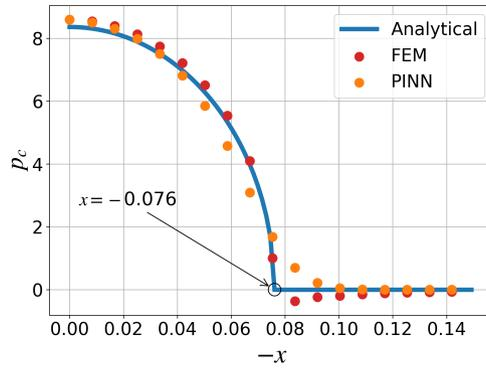
**Figure 15** Comparison of contact pressure distributions  $p_c(x)$  obtained by analytical solution, PINN and FEM for case 1.
