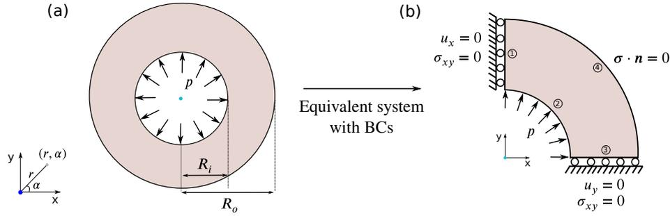
**Figure 9** The Lamé problem of elasticity. (a) The full problem under internal pressure, and (b) the equivalent problem due to the axisymmetrical nature of both geometry and loading, and accompanying boundary conditions.
