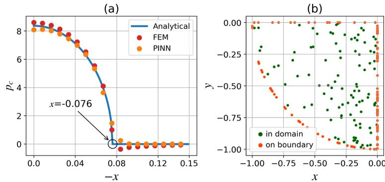
**Figure 16** Comparison of contact pressure distributions  $p_c(x)$  obtained by analytical solution, PINN and FEM for case 2. (a) PINNs as a data-enhanced forward solver, (b) distribution of data points generated through FEM simulations in the domain and on the boundary.
