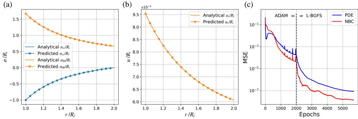
**Figure 10** Results for the Lamé problem of linear elasticity. (a) Comparison of normalized stresses obtained from the analytical solution and the predicted values, (b) comparison of normalized displacements, and (c) evolution of the MSE for the summed PDE loss and NBC loss.
