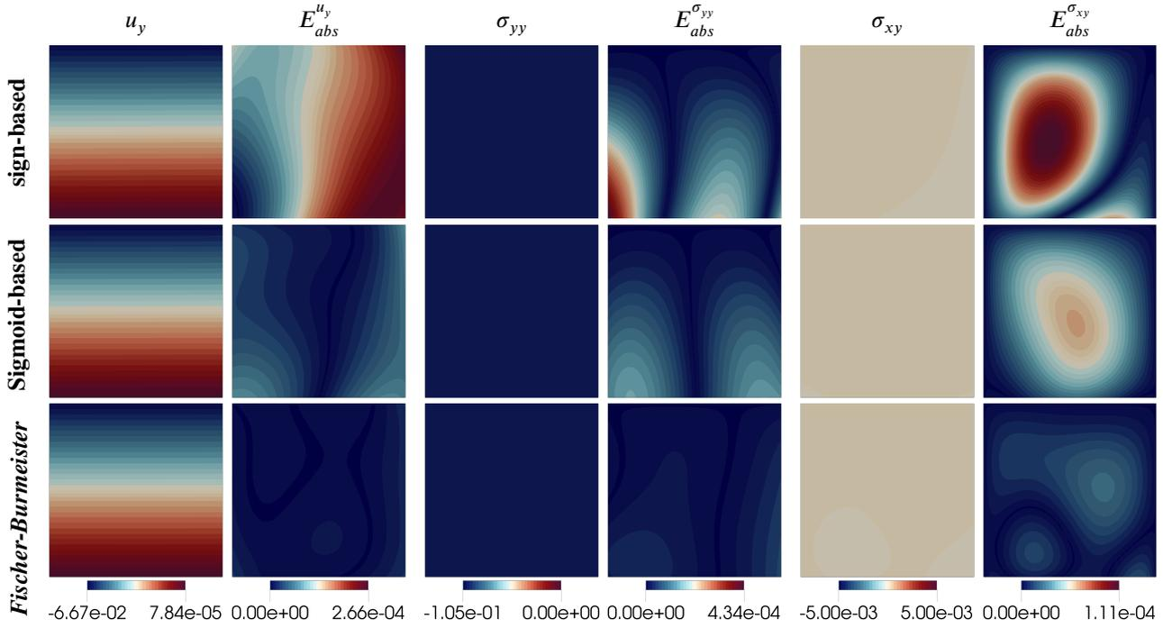
**Figure 12** Predictions of the displacement component  $u_y$ , stresses  $\sigma_{yy}$  and  $\sigma_{xy}$  with corresponding absolute errors  $E_{abs}^{u_y}$ ,  $E_{abs}^{\sigma_{yy}}$ ,  $E_{abs}^{\sigma_{xy}}$ . The contact constraints  $\mathcal{L}_{KKT}$  are enforced via three different methods: sign-based method, Sigmoid-based method and the *Fischer-Burmeister* NCP function. Absolute error  $E_{abs}^* = \text{abs}(* - *)$ .
