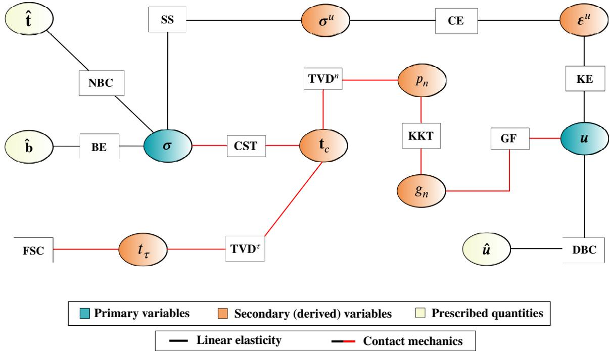
**Figure 2** Tonti's diagram of Hellinger–Reissner (HR) principle for contact problems with small strain theory and frictionless sliding condition.
