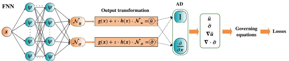
**Figure 4** Physics-informed neural networks in the mixed-variable form to solve quasi-static solid and contact mechanics problems without additional network parameters.
