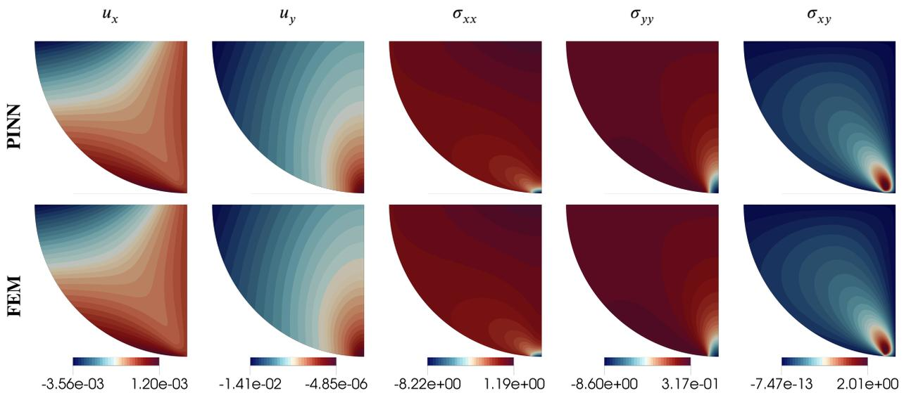
**Figure 14** PINNs as pure forward solver for the Hertzian contact problem. Comparison of stress and displacement components obtained by PINN and FEM.
