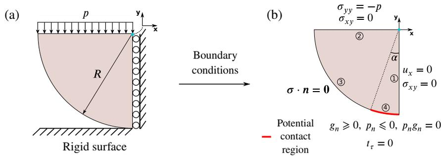
**Figure 13** The Hertzian contact problem between an elastic half-cylinder and a rigid flat surface (a) domain under uniform pressure on top and making use of symmetry, (b) accompanying boundary conditions.
