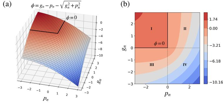
**Figure 7** The Fischer-Burmeister NCP function depending on gap  $g_n$  and contact pressure  $p_n$  as a 3D plot (a) and as a 2D contour plot (b).
