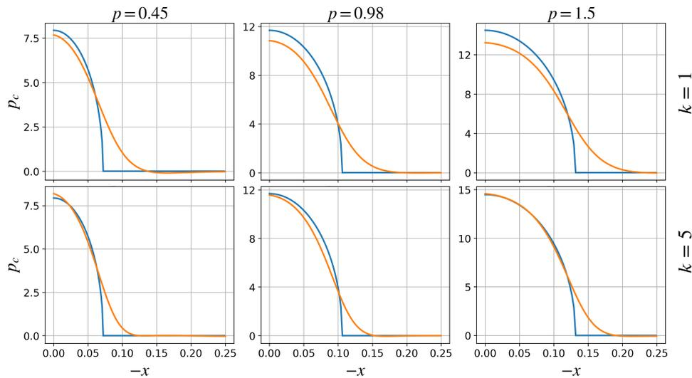
**Figure 19** Comparison of the contact pressure distribution obtained through a PINN-based surrogate model to the analytical solution. The PINNs are trained using different numbers of chunks.
