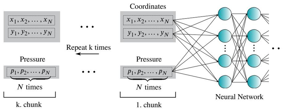
**Figure 18** An illustration of the procedure to include the applied external pressure as a neural network input.
