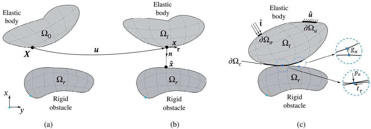
**Figure 1** Contact problem between an elastic body and a rigid obstacle. (a) Reference configuration, (b) current configuration, (c) accompanying boundary conditions, illustration of the gap  $g_n$ , tangential traction  $t_\tau$  and contact pressure  $p_n$ .
