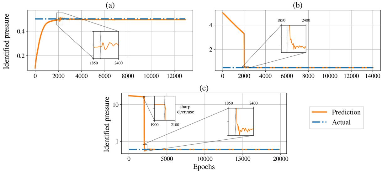
**Figure 17** Identification of the applied external pressure on the half-cylinder in case of different initial guesses (a)  $p_o = 0.1$ , (b)  $p_o = 5$ , (c)  $p_o = 20$ .
