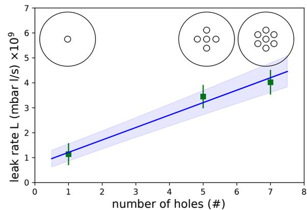
FIG. 5: Measured leak rate through the 2160 nm aluminised Mylar as a function of the number of 1-mm-diameter holes with a fitted straight line (blue) together with a shaded  $2\sigma$  confidence interval.
