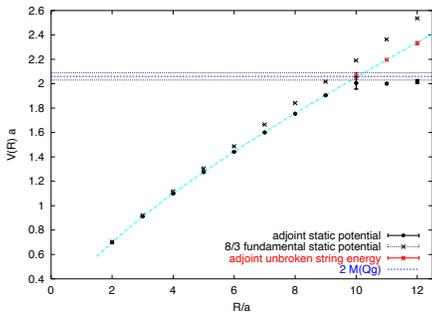
Figure 3: The adjoint and fundamental static potentials  $V(R)$  (the latter multiplied by the Casimir factor  $8/3$ ) versus  $R$  using Wilson loops only. The adjoint static potential remains approximately constant for  $R \geq R_b = 10a$  proving string breaking. The unbroken-string state energy is also drawn. The horizontal line at  $2.06(3)a^{-1}$  represents twice the mass of a glue lump. This is graph is from [60].
