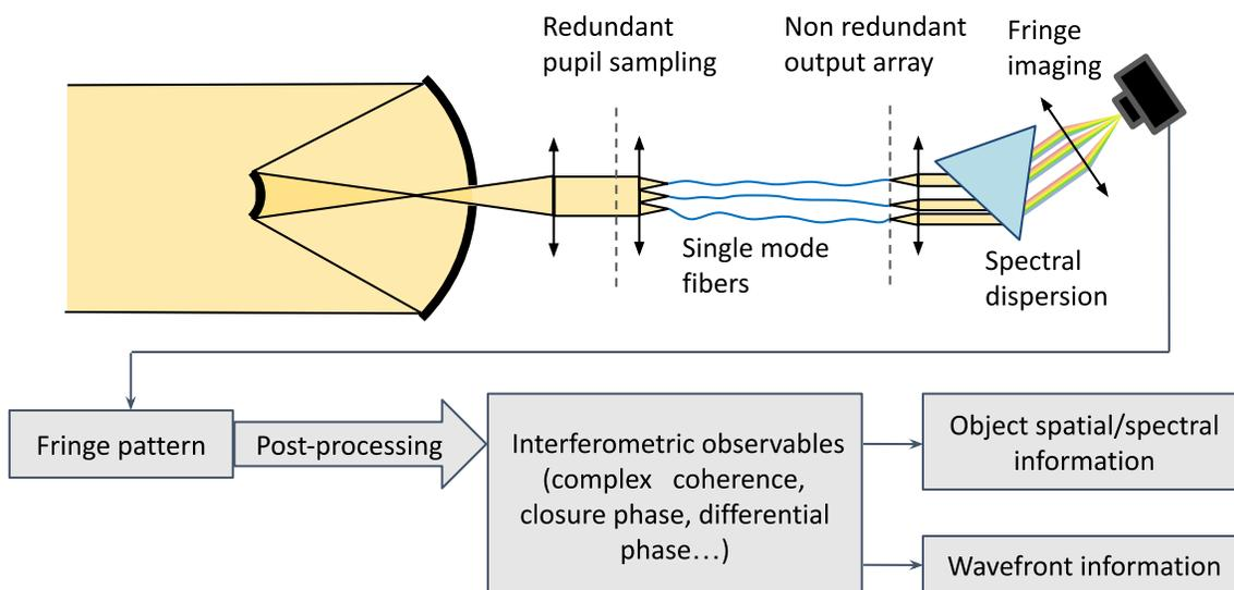
Figure 1. FIRST simplified principle. The pupil light is sampled thanks to a micro-lens array. The light from each sample, or subpupil is injected into a single-mode fiber. The single-mode fibers are rearranged into a 1D non-redundant array. Outputs of the fibers are dispersed and interfere on the science detector. Interferometric observables are extracted from the fringe pattern, allowing to obtain object's spatial/spectral information along with wavefront information.
