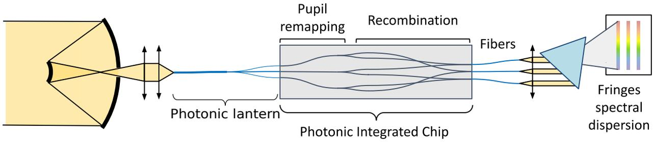
Figure 15. Instrument design with a photonic lantern feeding a photonic integrated chip.
