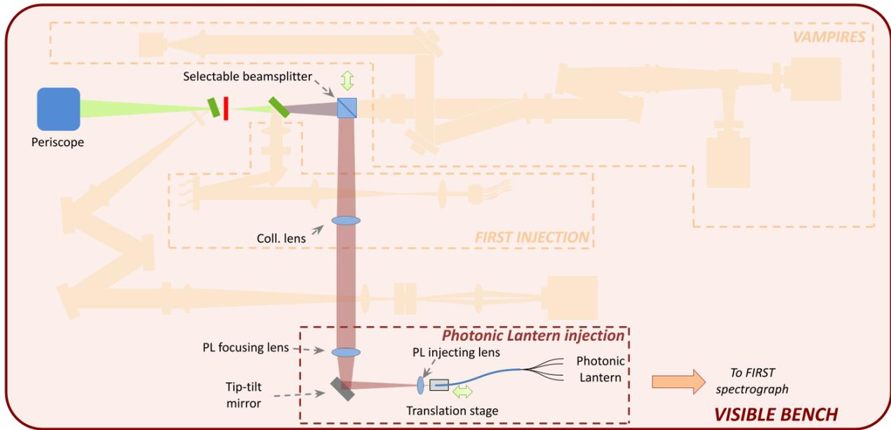
Figure 16. Photonic Lantern injection module on the SCExAO Visible bench.
