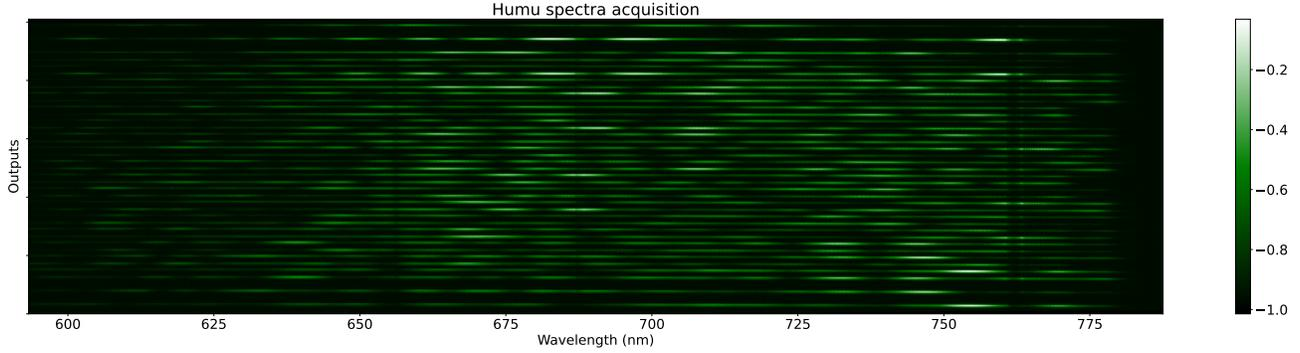
Figure 19. Spectra of Humu acquired with the Photonic Lantern. The horizontal axis is the wavelength dispersion, while the 38 output traces, corresponding to the two polarizations from each of the PL 19 SMF outputs, spread along the vertical axis.
