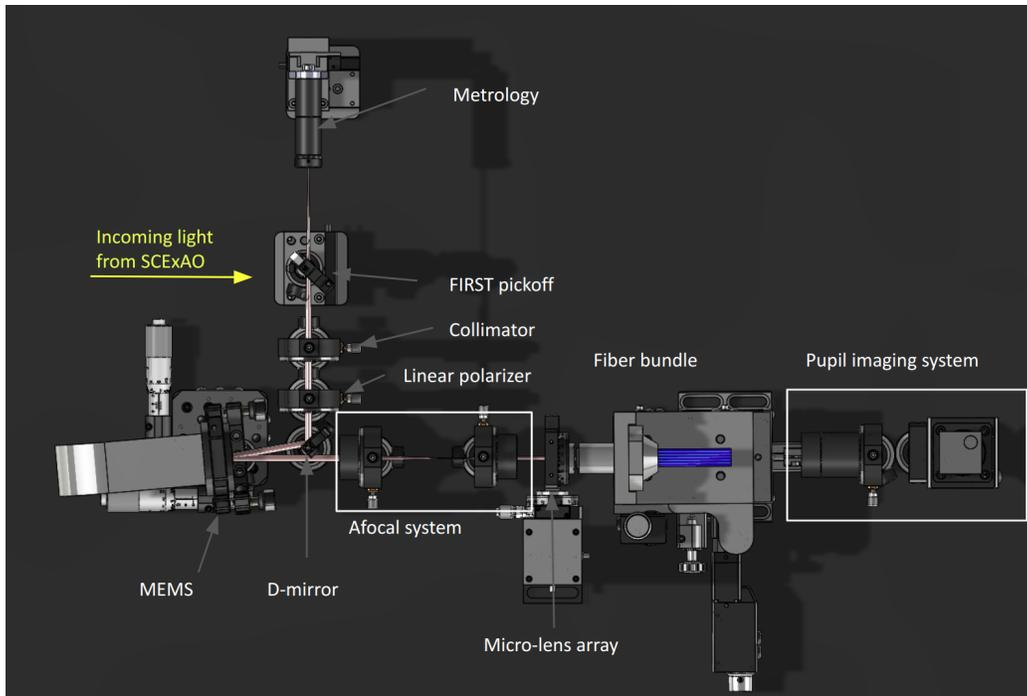
Figure 10. Upgraded FIRST injection module with a new MEMS, new optical setup including a D-mirror and a metrology source system.
