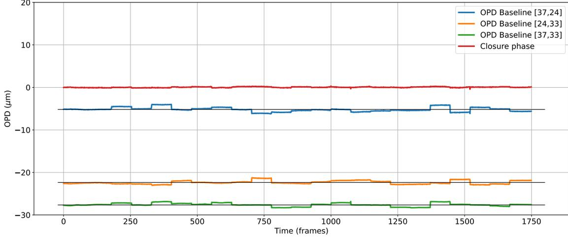
Figure 8. Evolution of the optical path difference for three baselines over time with petaling modes applied on SCEXAO DM.
