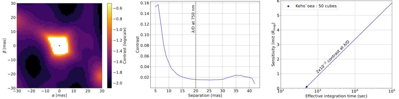
Figure 4. Performance of the FIRST instrument, estimated from unresolved source observation. Left :  $3\sigma$  detection map; Middle: Computation of the left map radial profile (excluding 0-values); Right: Extrapolation of the detection performance for different star magnitude as a function of the effective integration time.
