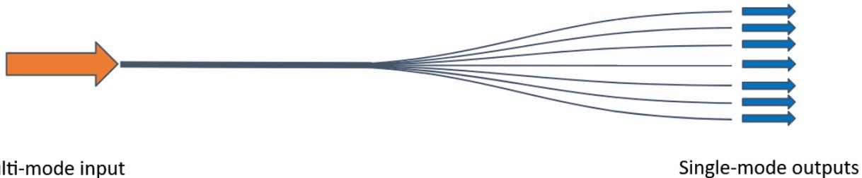
Figure 14. Principle of the pigtail photonic lantern approach: light is injected into a multi-mode input. The multi-mode waveguide slowly becomes several single-mode waveguides at the output.
