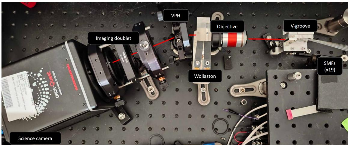
Figure 18. Spectrograph imaging the 19 SMF outputs of the photonic lantern.
