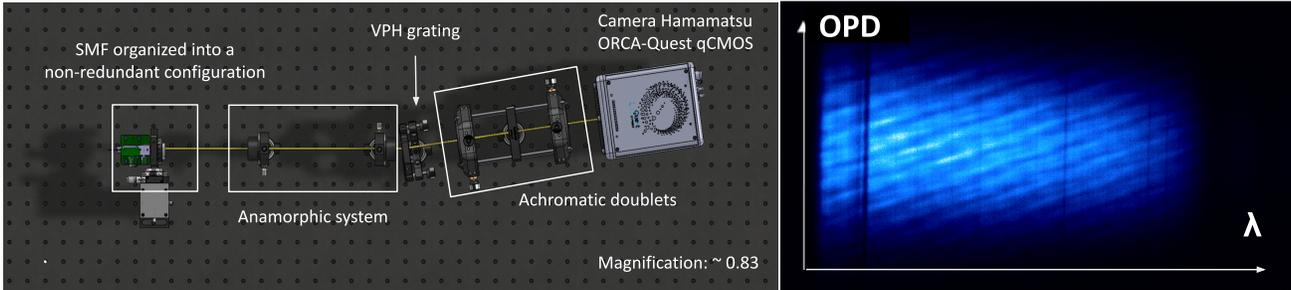
Figure 13. New R-4000 spectrograph integrated in FIRST. Left: CAD rendering of the FIRST anamorphic system followed by the spectrograph. Right: On-sky testing of the new spectrograph. Acquisition on Hōkūle'a [Arcturus]
