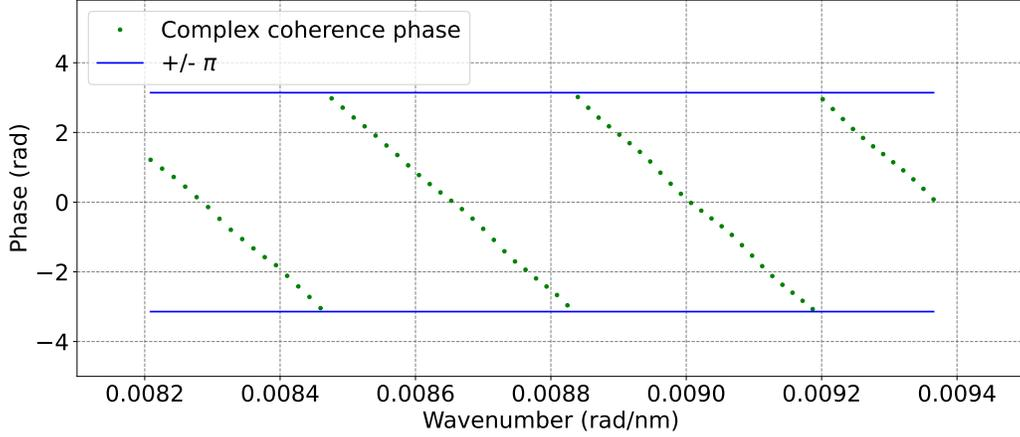
Figure 6. Phase of the complex coherence between subpupils linked to segments 37-24 as a function of the wavenumber defined as  $2\pi/\lambda$  (green). The phase is wrapped between  $\pm\pi$ , as materialized by the blue lines.
