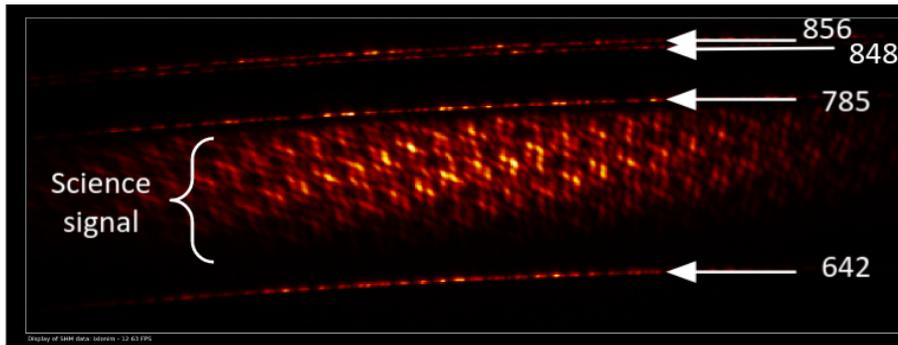
Figure 9. Raw image of the FIRST spectrograph where we image both the SCExAO calibration broadband laser (SuperK) and the FIRST internal metrology.
