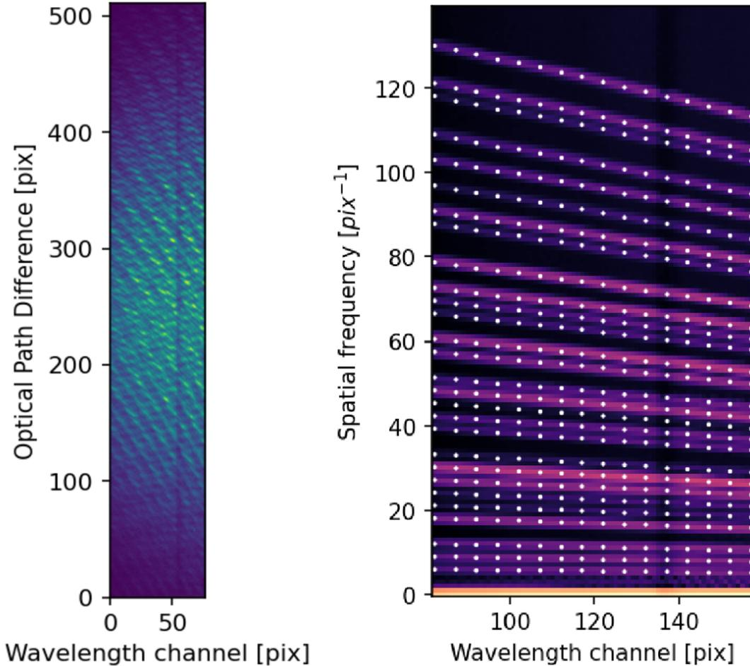
Figure 3. Typical image delivered by FIRST. Left: Exposure of 100 ms and 50 EMgain of Keho’oea, corrected from curvature. Right: Power spectral density computed from 30 cubes of 100 acquisitions with 100 ms exposure and 50 EMgain. The white dots show the PSD peak fitting for some selected wavelengths.
