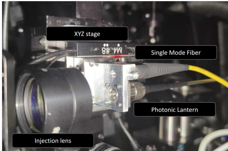
Figure 17. Injection module.
