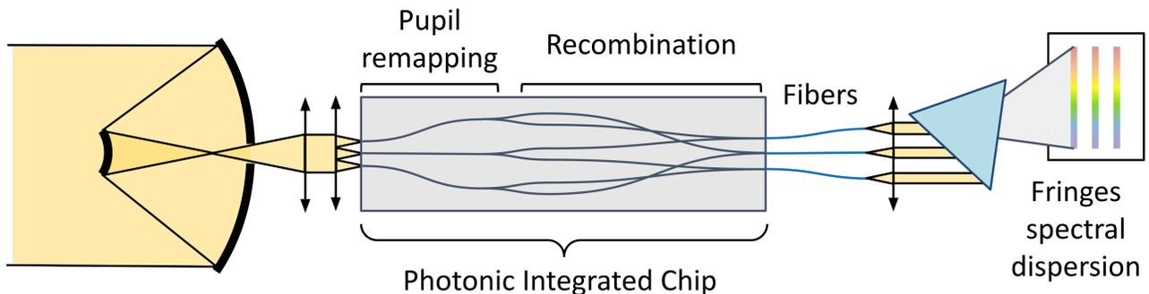
Figure 11. FIRST Photonic Integrated Chip approach principle.
