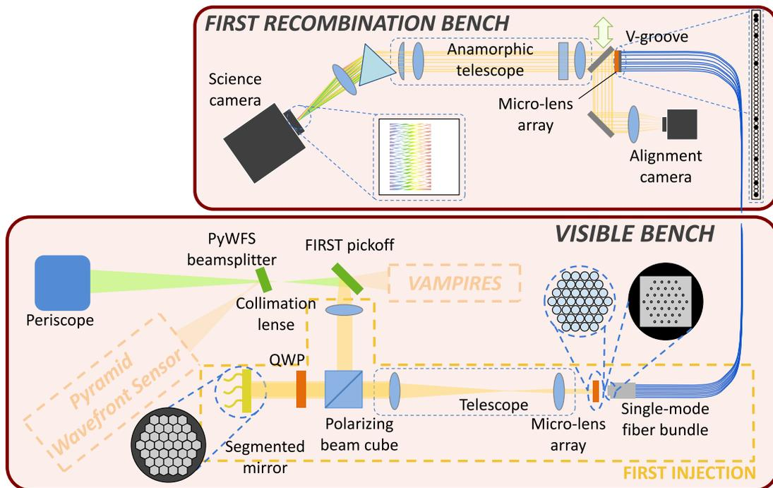
Figure 2. FIRST injection bench on the SCEXAO Visible bench (bottom), and FIRST recombination bench (top).
