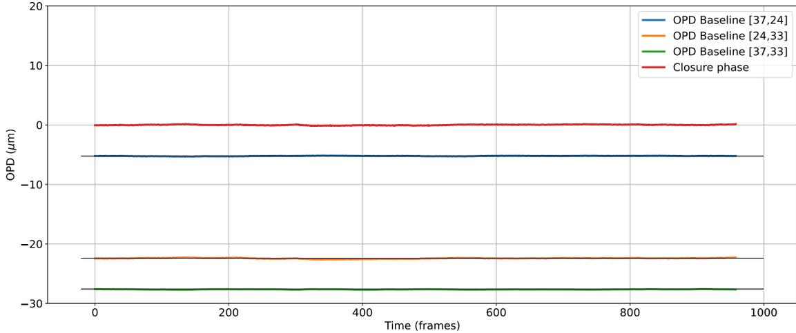
Figure 7. Evolution of the optical path difference for three baselines over time without petaling modes.
