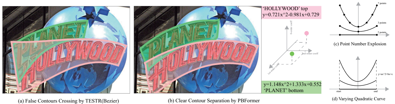
Figure 1: Advantages of PB over Bezier control points and polygon points. Comparing (a) and (b), PB divides adjacent texts more clearly than Bezier control points. (c) shows the number of output point increase gradually to represent shapes from straight to highly curved. (d) shows varying curve coefficients can handle dynamic shapes with fixed number of variables.
