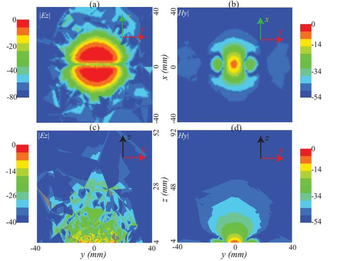
FIG. 5. The simulated  $E_z$  for (a) XY plane at a height of  $z = 4$  mm, (c) YZ plane with  $x = 0$ , and  $H_y$  at (b) XY plane at a height of  $z = 4$  mm, and (d) YZ plane with  $x = 0$ .
