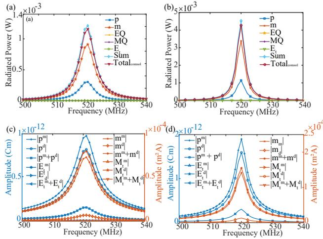
FIG. 2. Extracted radiated powers using Cartesian multi-pole expansion and numerically for vias separation of (a)  $s = 0.6$  mm and (b)  $1.2$  mm, while input impedance ranges from  $15k\Omega$  to  $150k\Omega$ , depending on  $s$ . Similarly, electric and magnetic dipoles evaluation on loop and dielectric disk separately for (c)  $s = 0.6$  mm and (d)  $s = 1.2$  mm.
