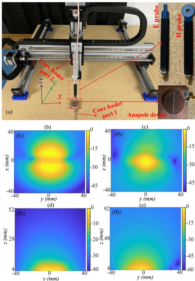
FIG. 6. (a) Automated measurement system along with used probes & the device and The measured  $E_z$  for (b)  $XY$  plane at a height of  $h = 4$  mm, (d)  $YZ$  plane with  $x = 0$ , and  $H_y$  for (c)  $XY$  plane at a height of  $h = 4$  mm, and (e)  $YZ$  plane with  $x = 0$ .
