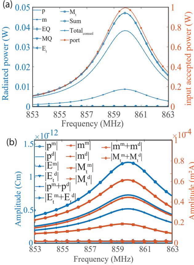
FIG. 4. (a) Cartesian multi-pole expansion and numerical evaluation for radiated and accepted powers, and (b) contribution assessment of the metallic and dielectric parts for electric and magnetic dipoles.
