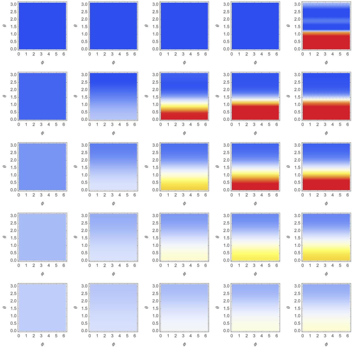
Figure 2: Simulation of the heat transfer from (31) with  $\alpha = 1, M = 5$ . Horizontally, we have fields on five different layers; vertically, the time goes from top to bottom in steps  $t_i = 0, 0.2, 0.4, 0.6, 0.8$ . It can be seen that the heat initially positioned close to a pole of the outermost layer slowly dissipates across all layers and moves toward thermal equilibrium.
