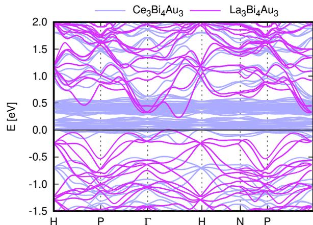
FIG. 9. Band-structures of  $Ce_3Bi_4Au_3$  (light blue) and  $La_3Bi_4Au_3$  (magenta; see also Ref. [14]) within DFT: The system is insulating (metallic) in the absence (presence) of the  $4f$ -electron—in direct opposition to the related pair of materials  $RE_3Bi_4Pt_3$  ( $RE=Ce, La$ ) [4].
