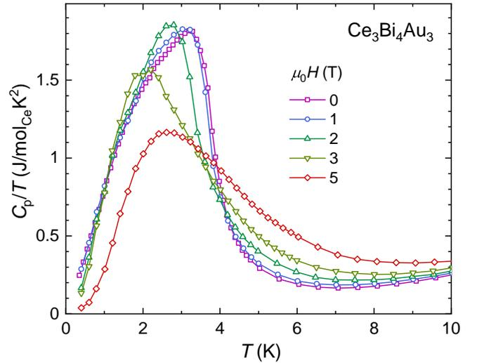
FIG. 4.  $C_p/T$  vs.  $T$  of  $\text{Ce}_3\text{Bi}_4\text{Au}_3$  measured under different applied magnetic fields.
