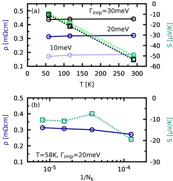
FIG. 10. Simulated resistivity and Seebeck coefficient: (a) dependence on the added impurity scattering rate (light to dark:  $\Gamma_{\text{imp}} = 10, 20, 30$  meV); blue: resistivity  $\rho$ ; green: Seebeck coefficient  $S$ . (b) convergence of  $\rho$  and  $S$  with the Brillouin zone discretization ( $N_k$ : number of reducible  $\mathbf{k}$  points). The calculations in Fig. 7b use the finest mesh ( $N_k = 50^3$ ).
