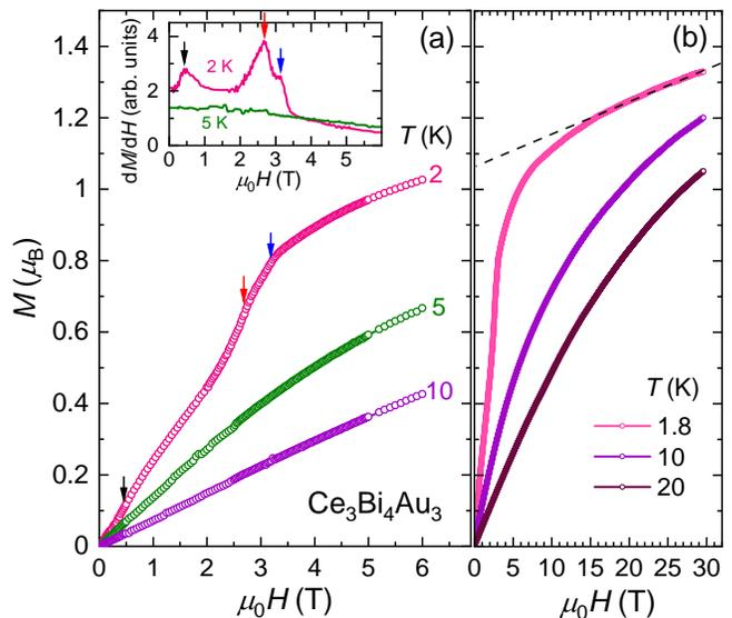
FIG. 2. (a) Magnetization of  $\text{Ce}_3\text{Bi}_4\text{Au}_3$  versus applied magnetic field, measured at different temperatures. The derivative  $dM/dH$  is plotted in the inset. Various features in  $M(H)$  are indicated by the arrows. (b) High-field magnetization measured at several temperatures.
