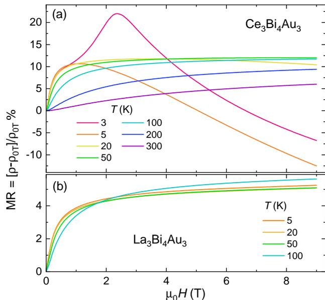
FIG. 8. Transverse Magnetoresistance  $MR = [\rho - \rho_{0T}] / \rho_{0T}$  as a function of magnetic field measured at different temperatures for (a)  $Ce_3Bi_4Au_3$  and (b)  $La_3Bi_4Au_3$ .
