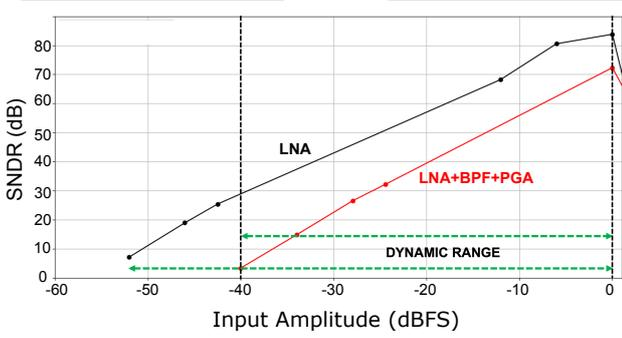
Fig. 7: SNDR Measurement of an AFE Channel.
