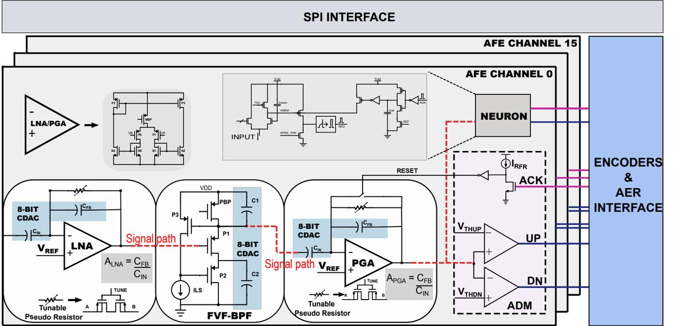
Fig. 3: Architecture of SPAIC Analog Front-End ASIC.
