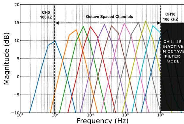
Fig. 6: Frequency Response of the bandpass filter bank
