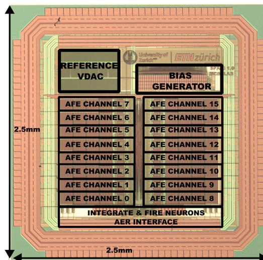
Fig. 2: SPAIC chip micrograph.
