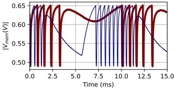
Fig. 9: Neuron's membrane potential response for different amplitudes of the input signal of the AFE. Red (100mV), Blue (400mV).
