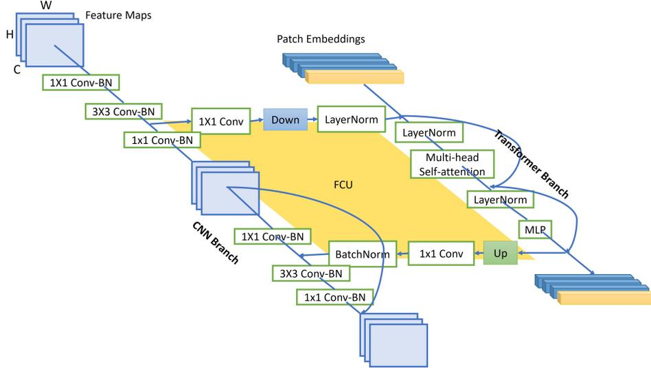
**Fig. 8:** Conformer architecture which leverages both local features provided by CNNs and global features provided by transformers in Feature Coupling Unit (FCU) (figure from [58]).
