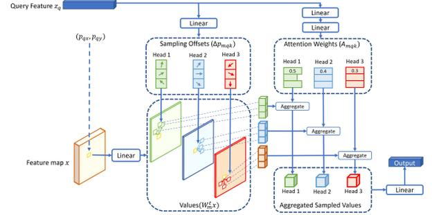
**Fig. 6:** The block diagram for the Deformable attention module.  $z_q$  is the content feature of the query,  $x$  is the feature map and  $p_q$  is the reference point in 2-D grid. In short, the deformable attention module only attends to a small set of key sampling points around the reference point (different in each head). This significantly reduces the complexity and further improves the convergence (figure from [41]).
