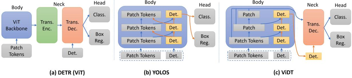
**Fig. 7:** ViDT (c) mixes DETR (with ViT backbone or other fully transformer-based backbones) (a) with YOLOs architecture (b) in a multi-scale feature learning pipeline to achieve SOTA results (figure from [42]).
