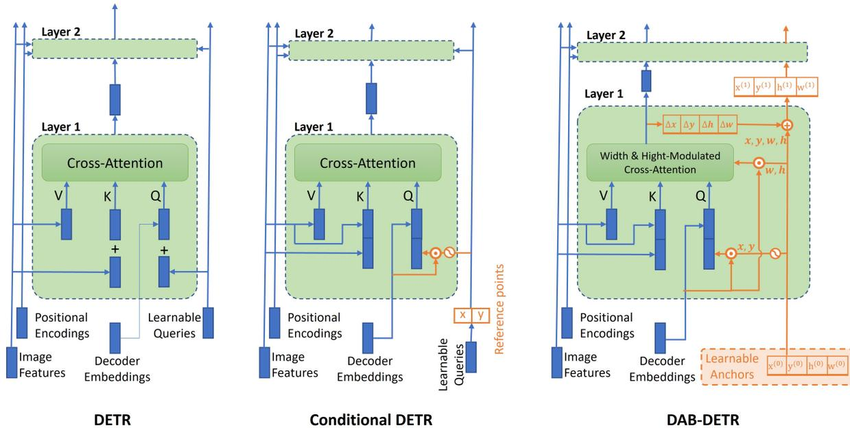
**Fig. 9:** DAB-DETR improves Conditional DETR and utilizes dynamic anchor boxes to sequentially provide better reference query points and anchor sizes (figure from [67]).
