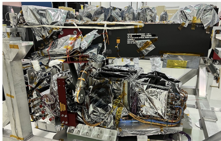
Figure 2. The optical bench mounted above the EHTS shortly after integration; wiring between the control electronics and optical components had not yet been installed. The optical elements are covered with protective tents for contamination control.
