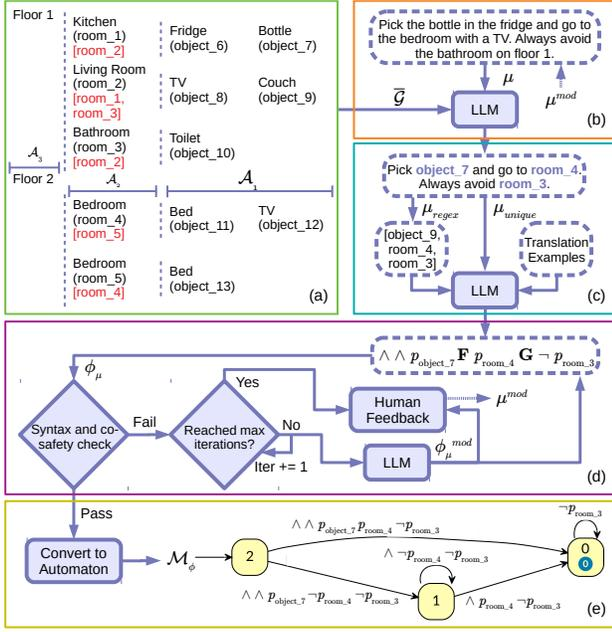
Fig. 2: Natural language to LTL translation. (a) Attribute hierarchy  $\bar{\mathcal{G}}$ . The unique IDs and the room connections are shown in parenthesis and inside red brackets, respectively. (b) Unique ID extraction from natural language mission  $\mu$ . (c) LTL formula generation from natural language specification. (d) Syntax and co-safety check over the generated LTL formula  $\phi_\mu$ . (e) Automaton construction.
