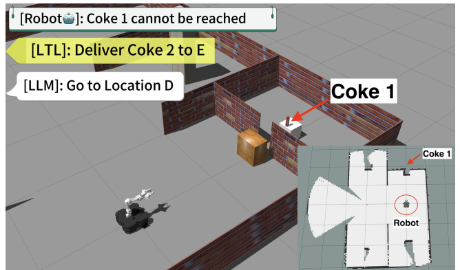
Fig. 5: Reacting to Infeasible Sub-tasks: As the robot navigates towards Coke 1, it builds the occupancy grid map of the environment allowing it to realize that Coke 1 is not accessible. Once this happens, the robot asks for help from the LTL planner.
