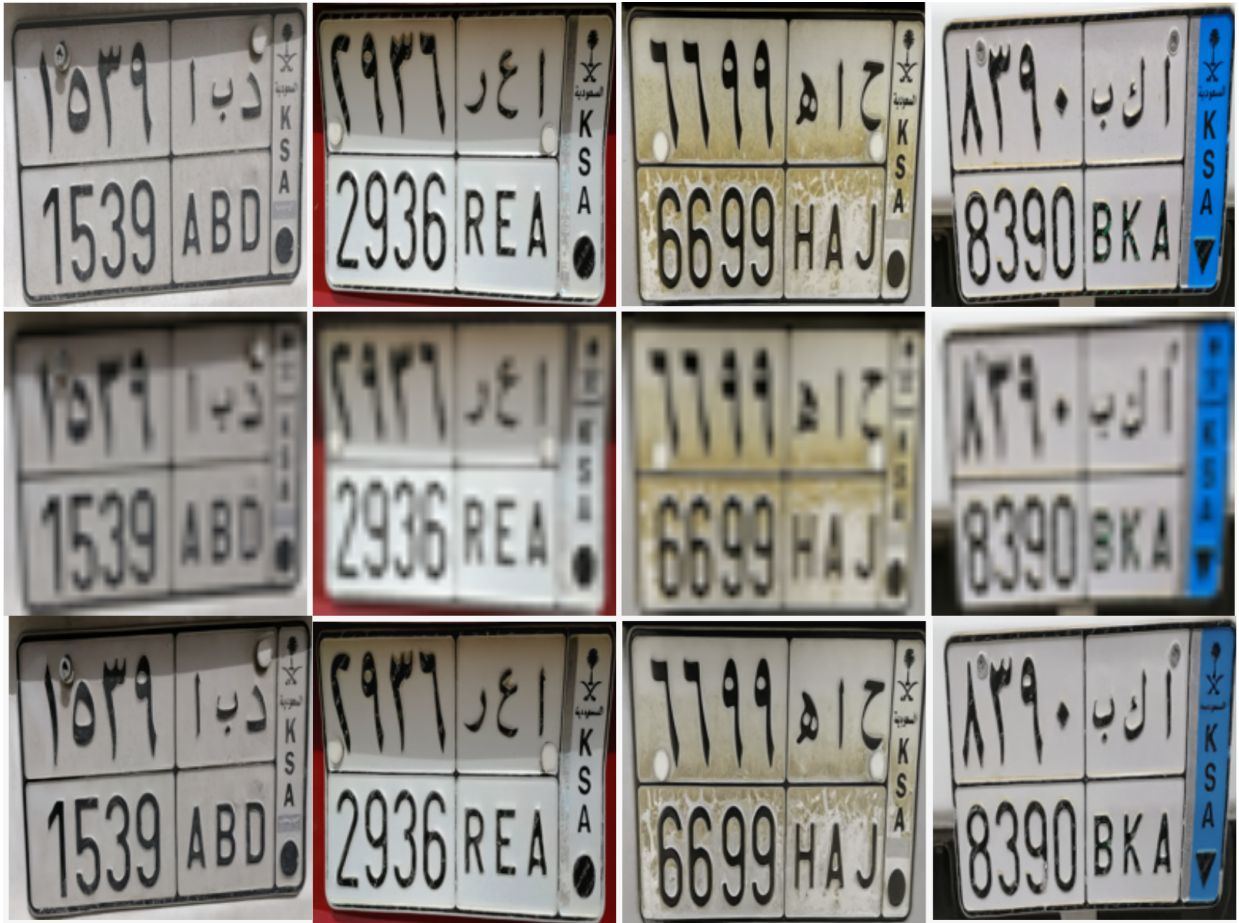
Fig. 5: First top row has the original HR image of (192 \times 192) resolution. Middle row has the downsampled LR image of (48 \times 48) resolution. Last row (bottom) has the super resolved images using diffusion model with (192 \times 192) resolution.
