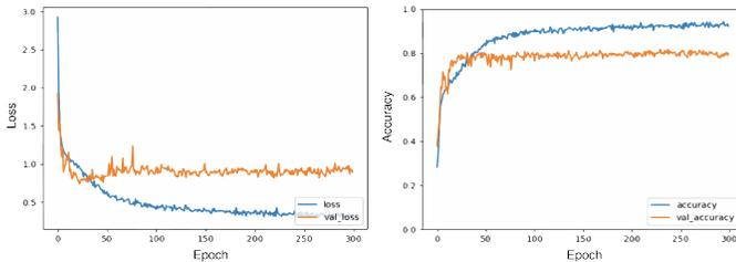
Fig. 6: Loss and accuracy of proposed model
