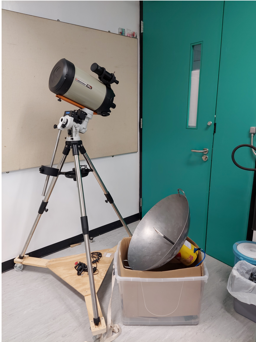
Figure 1: Overview of the 61.0 cm aperture WTH radio telescope (bottom right), compared with a 20.3 cm Schmidt-Cassegrain optical telescope along with the mount from Celestron (top left). The WTH system is temporarily ‘mounted’ on a plastic storage box with wheels for easier transporting the system to observation site.
