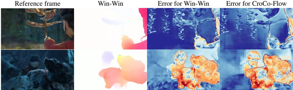
Figure 4: **Example result on Spring test set.** For the error maps, blue and red denote low and high errors, respectively. *Block artefacts* are clearly visible for CroCo-Flow but notably absent for Win-Win.
