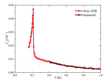
FIG. 7. Temperature dependence of the total (magnetic) heat capacity of the NaYbGeO<sub>4</sub>-based ADR pellet determined from the warming curve shown in Fig 6 by calculating  $C_{\rm ADR} = \dot{Q}/\dot{T}$  (red points). The constant heat input  $\dot{Q} = 0.58 \mu \rm W$  was used to obtain agreement with the measured heat capacity (black points) above 0.4 K.
