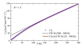
FIG. 3. Inverse magnetic susceptibility  $1/\chi$  vs. temperature of NaYbGeO<sub>4</sub> at a field of 1 T. Dashed and solid lines represent the fits by Eq. 1 and Eq. 2, respectively.
