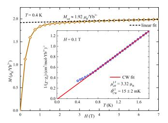
FIG. 4. Isothermal magnetization M(H) of NaYbGeO<sub>4</sub> at a temperature of 0.4 K. Dashed line represents linear contribution (see text). The inset shows the low-temperature inverse magnetic susceptibility after subtracting  $\chi_0$  along with the CW fit.
