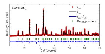
FIG. 2. Powder x-ray diffraction pattern (open red circles) for NaYbGeO $_4$  at room temperatures. The solid line represents the Rietveld refinement, with the vertical bars showing the expected Bragg peak positions and the lower solid blue line representing the difference between observed and calculated intensities.
