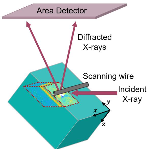
**Figure S-2:** A schematic of the DAXM measurements showing the coordinates used in this study, the relative position of the indent, the scanned volume (dashed red lines), the bulk sample, and the beamline set-up. The example data shown here is from the Fe10Cr irradiated sample. The relative size of the scanned volume and the bulk sample is not to scale.
