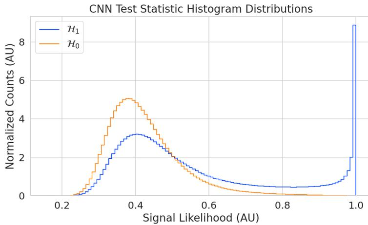
**Figure 8:** Histograms of the trained CNN model output from the test dataset. The blue histogram shows the model outputs for signal data. The oddly shaped peak near the end is the result of the softmax function mapping the long tail of the raw output distribution to the range  $[0, 1]$ .
