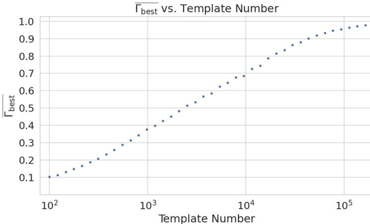
**Figure 7:** The mean match of the matched filter template bank to a test set of randomly parameterized signals as a function of the number of templates. The parameter space includes pitch angles from  $85.5 - 88.5^\circ$  and energies from  $18575 - 18580$  eV.
