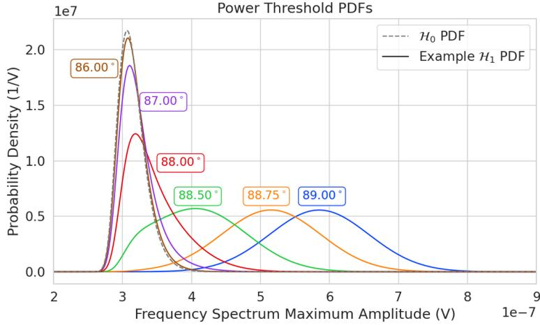
**Figure 5:** PDFs of the power threshold test statistic for CRES signals with various pitch angles as well as the PDF for the noise-only ( $\mathcal{H}_0$ ) case. As the pitch angle is decreased the  $\mathcal{H}_1$  PDFs converge towards the noise PDF, which indicates that the power threshold is unable to distinguish between signal and noise.
