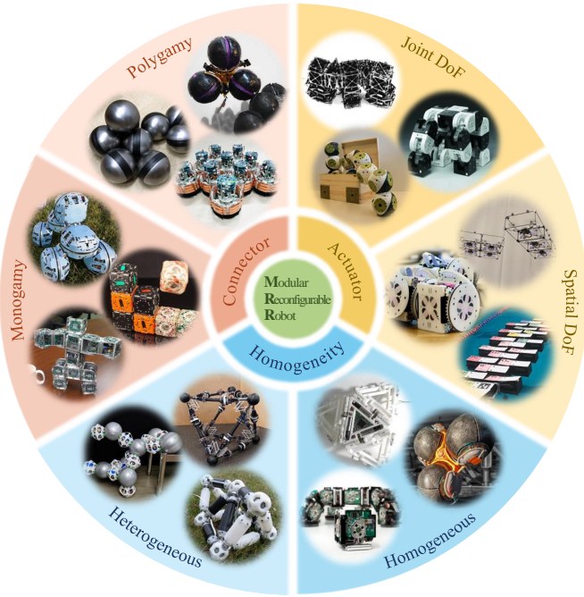
Fig. 3. A novel tripartite framework decodes MRR systems into three elements: connectors, actuators, and homogeneity. The classification of these three elements differs at various levels: connectors are classified based on the degree of the connection topology they form, actuators are classified by the type of DoF they provide, and homogeneity pertains to the system’s classification based on its constitution, determining whether it contains a single type or multiple types of modules. Representative MRRs are provided for each element attribute.
