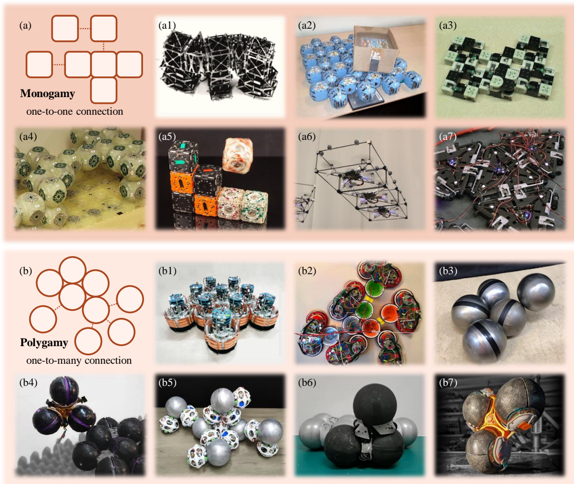
Fig. 4. Connector elements are categorized as either (a) monogamy or (b) polygamy. Monogamous connectors establish one-to-one relationships among connectors. Noteworthy exemplars encompass: (a1) Polypod [26], (a2) ATRON [42], (a3) M-TRAN [30], (a4) Soldercubes [53], (a5) M-Blocks [54], (a6) ModQuad [35], and (a7) Mori3 [21]. In contrast, polygamous connectors create one-to-many relationships among connectors. Illustrative instances encompass: (b1) Slimebot [33], (b2) FireAnt2D [55], (b3) FreeBOT [51], (b4) FireAnt3D [7], (b5) FreeSN [8], (b6) SnailBOT [13], and (b7) FireAntV3 [52].
