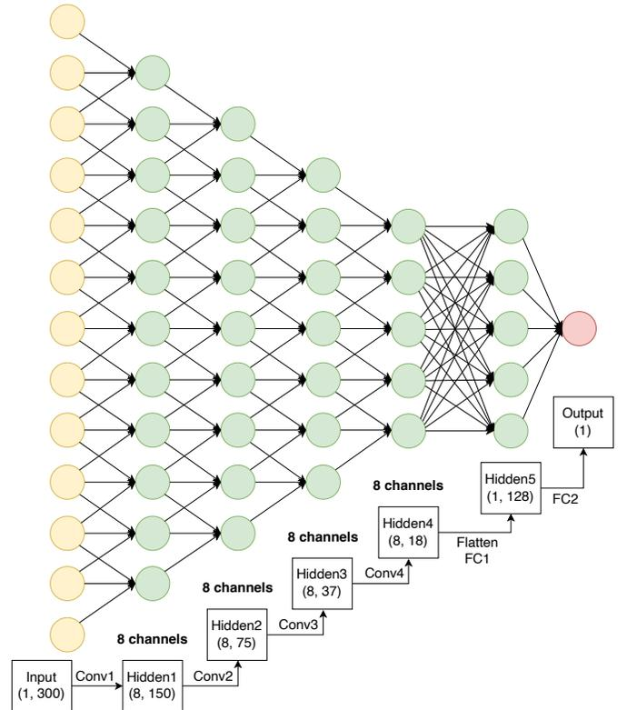
**Figure 6.** Schematic diagram of the CNN-based RegNet architecture, which is designed to extract redshifts from *Gaia* DR3 BP/RP spectra. This diagram shows the process of a single spectrum with 300 points passing through the network and yielding the redshift value. For simplicity, only a small fraction of the input and hidden neurons are plotted.
