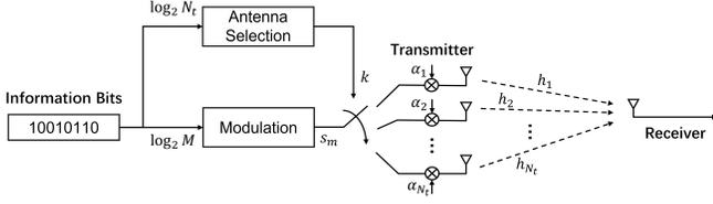
Fig. 1: Block diagram of SM transmitter with pre-scaling.
