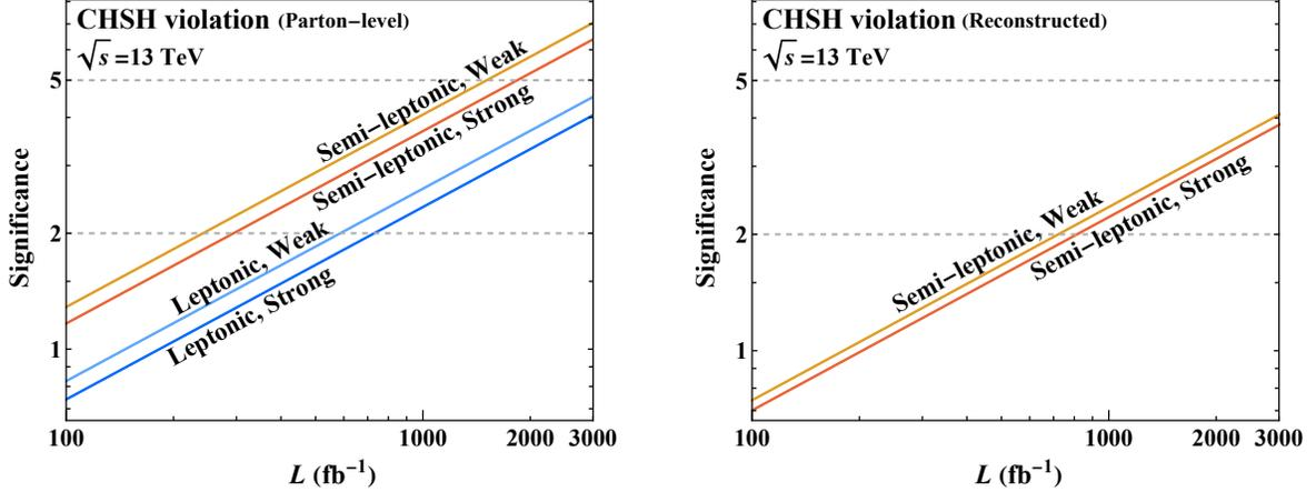
**Figure 10:** Expected significance of CHSH violation detection as a function of the integrated luminosity at the 13 TeV LHC at parton-level (left) and after detector simulation, reconstruction, and parametric fitting (right).
