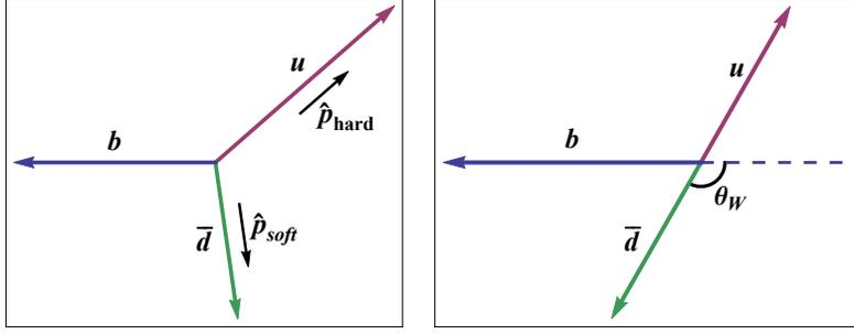
**Figure 2:** Illustration of the top decay system in the rest frame of the  $t$  (left) and rest frame of the  $W$  (right). Between the down-type anti-quark and the up-type quark in the  $t$  rest frame, the down-type anti-quark tends to be softer while the up-type quark tends to be harder.
