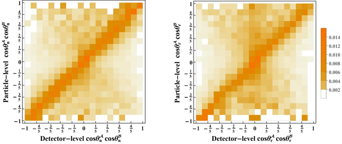
**Figure 12:** Response matrix of  $\cos \theta_n^A \cos \theta_n^B$  (left) and  $\cos \theta_r^A \cos \theta_r^B$  (right) computed at  $\sqrt{s} = 13$  TeV. Parton-level events have signal region cuts and no event selection, while detector-level events include detector effects and the effects of event selection described in Sec. 4.2.
