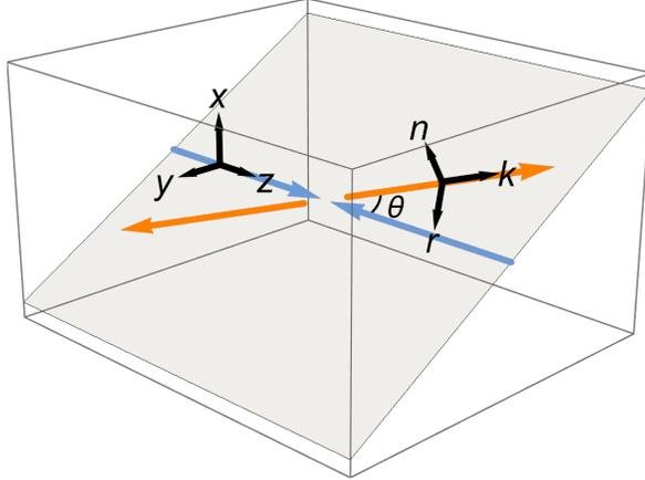
**Figure 1:** Illustration of the fixed beam basis  $\{\hat{x}, \hat{y}, \hat{z}\}$  and the helicity basis  $\{\hat{r}, \hat{k}, \hat{n}\}$ . The incoming beams are blue and the outgoing top and anti-top are orange.  $\theta$  is the polar angle between the  $\hat{z}$ -axis (the beam direction) and the  $\hat{k}$ -axis (the top quark momentum direction).
