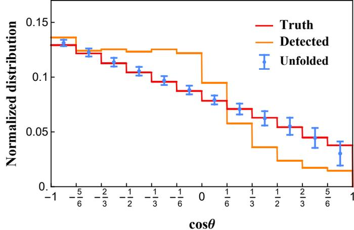
**Figure 13:** Differential decay width of the top quark at parton-level (red), uncorrected detector-level (orange), and after unfolding (blue markers).
